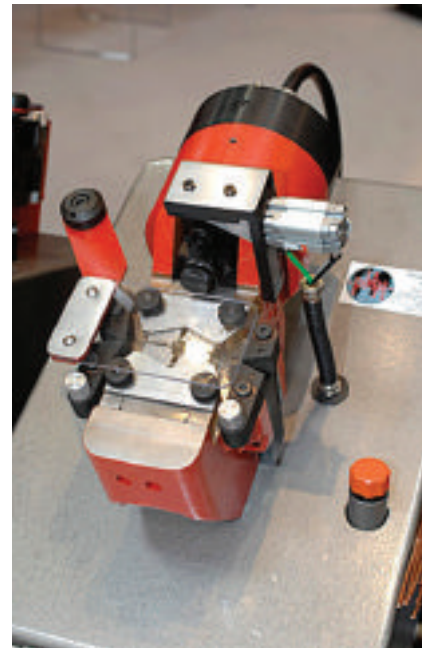
▲ The welding head of the new HP100 auto air/hydraulic cold welder from Pressure Welding Machines, launched at Dusseldorf's wire 2008
