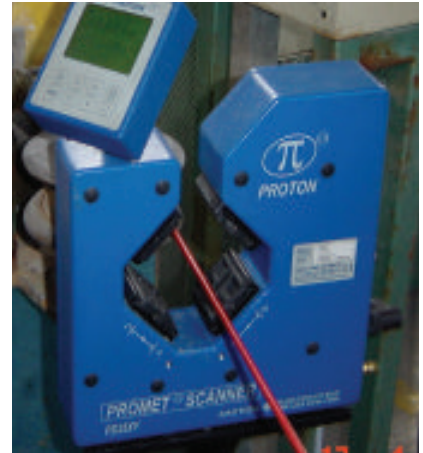
▲ InteliSENS (Intelligent Sensor) measurement gauge from Proton Products can be found in cable making facilities around the world
