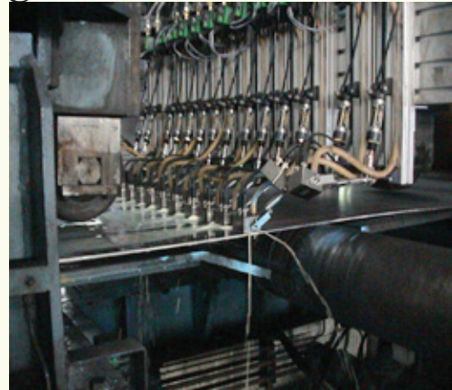
ERW mill 1900 mm coil - Thickness 4-16 mm
