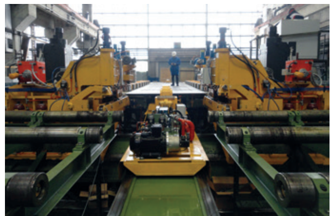
Figure 3: Edge milling machine 18"-56". Client: Hunan Shengli, China, 2013
