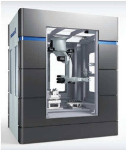
The LoadMaster Assist enables lights-out shifts for turning and milling centres
