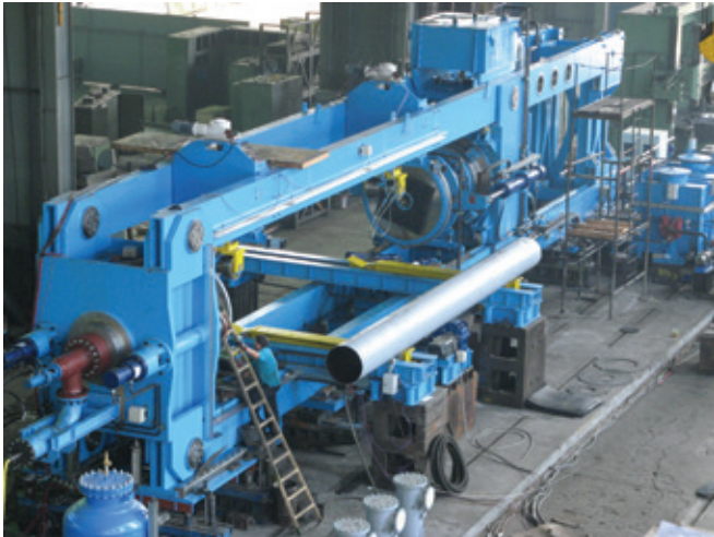
Figure 4: Pipe hydrotester 16"-60". Client: Essar Hazira, India, 2010
