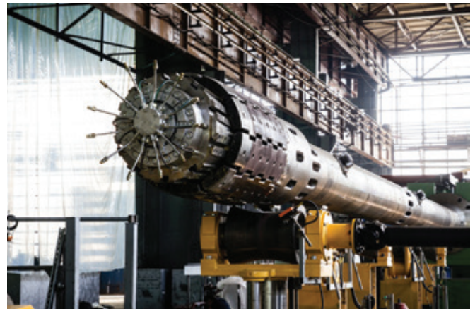
Figure 2: Mechanical expander 18"-56". Client: Hunan Shengli, China, 2013
