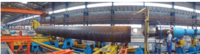
Figure 1: Mechanical expander 16"-60". Client: ESSAR Hazira, India, 2010
