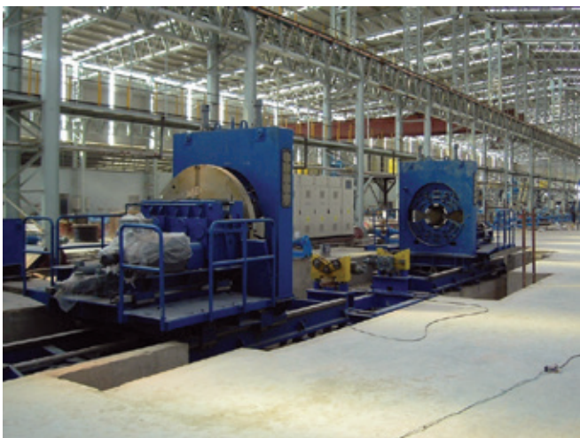
Figure 5: Facing and bevelling machine 16"-56". Client: Man Anjar, India, 2005
