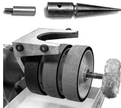
Shown on Genie: adaptor, tapered spindle and buff.
