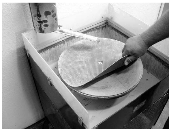
Magnetic Novas are easy to exchange.
