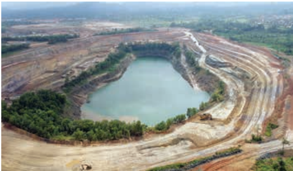
Mining operations around the old Nkran pit, which is currently being dewatered (photo: Asanko Gold).
