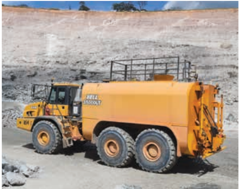
ADTs can easily be adapted to a variety of roles. This 35 000 litre water tanker is working at an emerald mine in Zambia (photo: Arthur Tassell).
