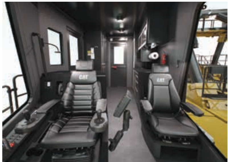
The well-appointed cab of a Cat rope shovel.
