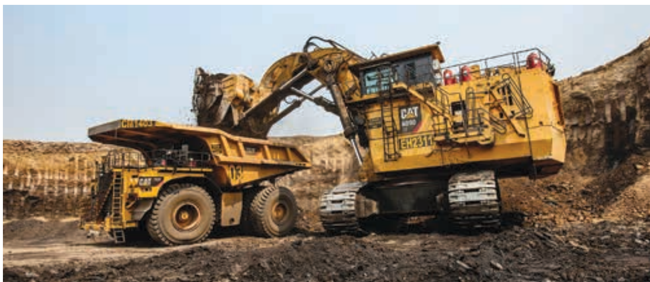
A Cat 6090 FS shovel loads a Cat 797F ultra-truck at the Moatize coal mine in Mozambique.
