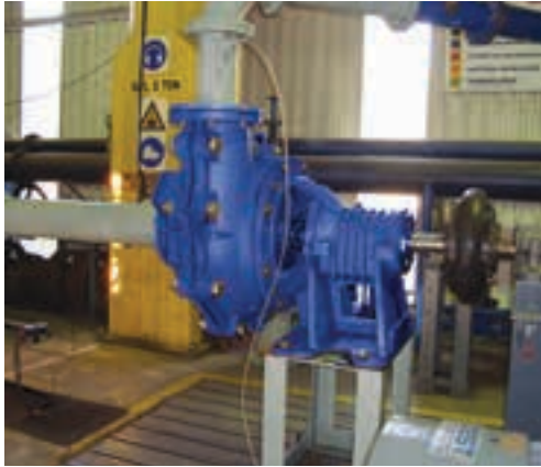
The Warman WBH slurry pump undergoing testing at Weir Mineral Africa's Alrode manufacturing centre.
