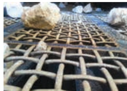
FLSmith has designed a hybrid poly wire modular panel for use in Rietvlei silica mine's screening process.
