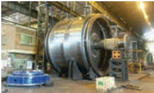
DCD Heavy Engineering is nearing completion of man and rock winder build for a Zambian mine. The rock winder – measuring 7.2 m in diameter and weighing 175 t when assembled – collects rock from depths of up to 2.0 km.
