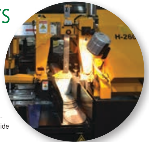
An Everising bandsaw machine being demonstrated cutting a batch of 3.0 mm discs off a 120 mm round bar. Automatic clamping between cuts and accurate forward-feed allows for continuous cutting of an exact number of discs.
