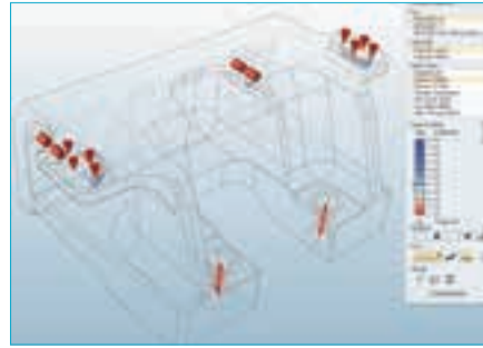
Defining supports and loads prior to the analysis with solidThinking Inspire.
