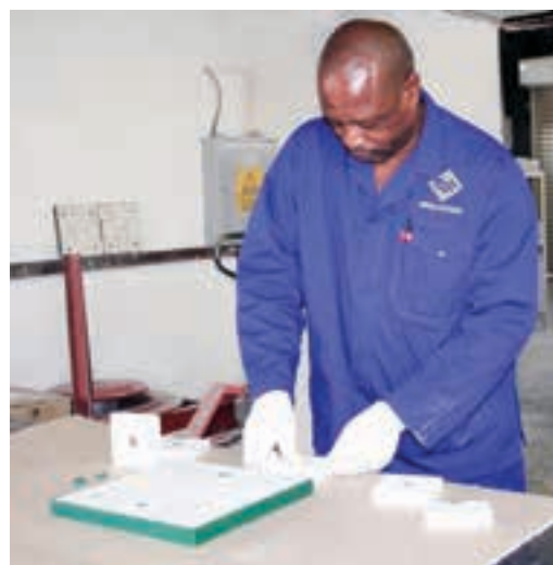
Multotec Wear Linings' senior assembler, Simon Ndlovu assembling Multotec Green Dot Tiles into a Quick Fit Panel.
