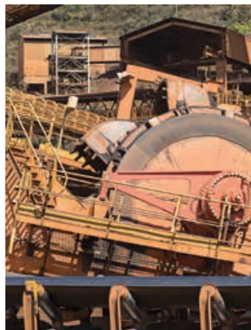
The use of Hägglands direct drives on bucket wheel stacker/reclaimers enables avalanches to be overcome more easily. This has led to these drives being specified on all of Vale's new and retrofit bucket wheels.
