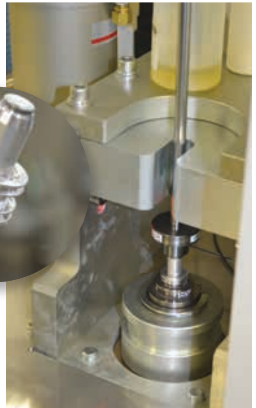
Left: Thread rollers are used to generate the tie rod and piston rod threads.
