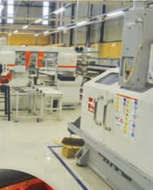
Left above: Materials come into the factory and go directly into bulk storage. Stroke related parts are cut using cutting machines on receipt of a customer order.
