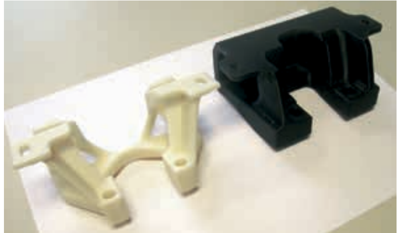
Model of the 3D printed version of the anti roll system support.
