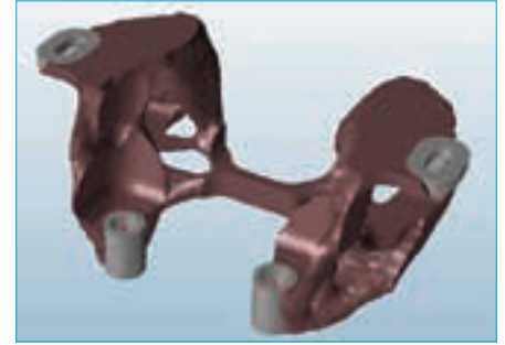
Result of the topology optimisation with solidThinking Inspire.
