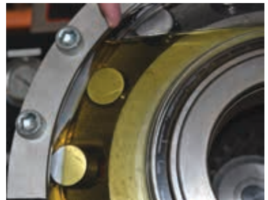
Hägglunds direct drive hydraulic motors have a fixed circumferential cam. Under hydraulic pressure, radial pistons with end rollers push against this cam causing the inner to rotate.
