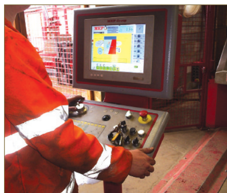
○ The operator station for the stirrup bender
