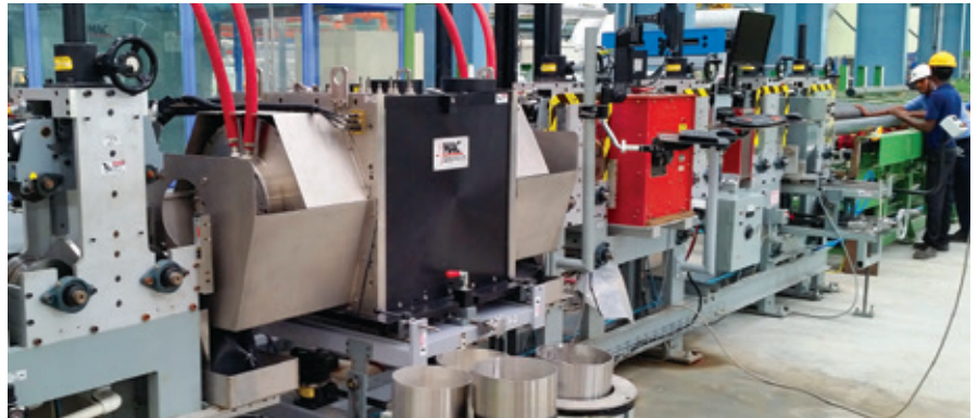
The Echomac ultrasonic rotary tester is part of the MAC Multi-Test system
