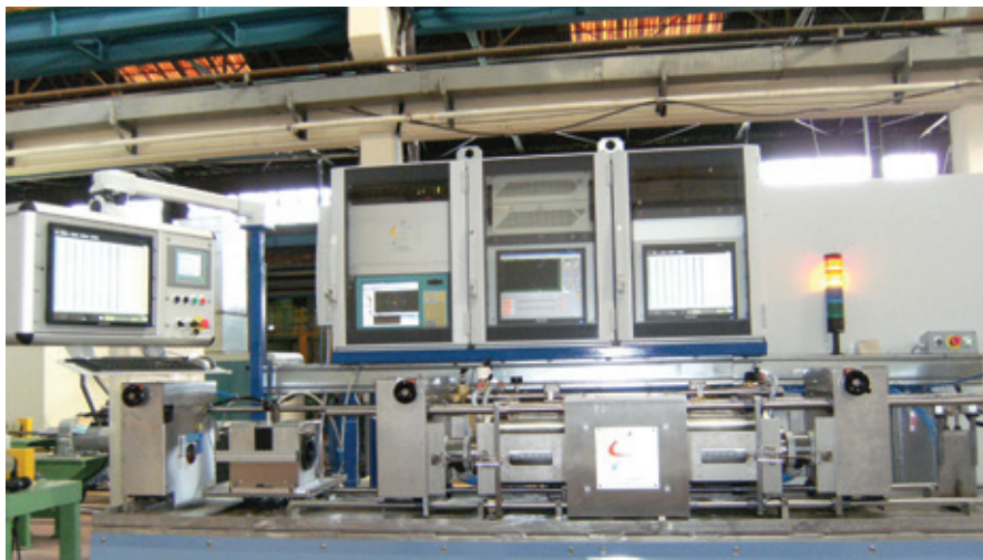
Complete titanium tube inspection by ultrasonic and eddy current testing
