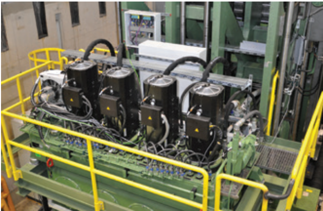
Beisteel's new JCO pipe forming press is equipped with a variable-speed pump control system
