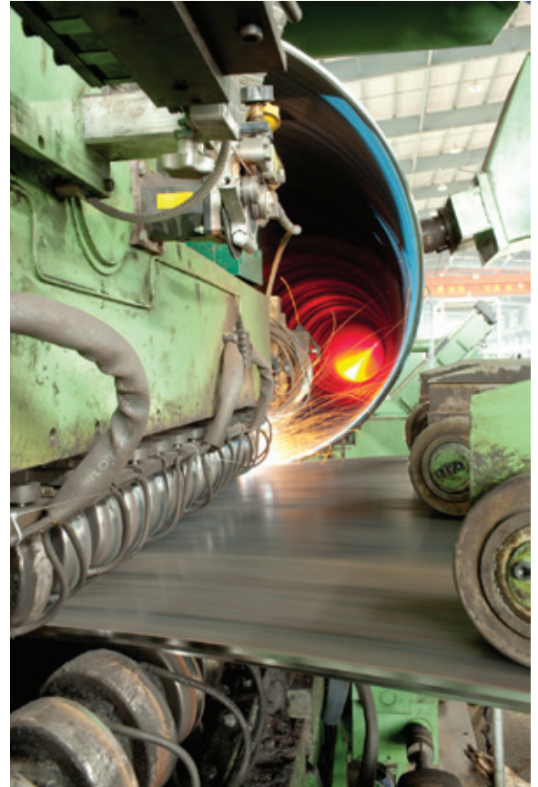
Shaping and high-speed tack welding of a pipe
