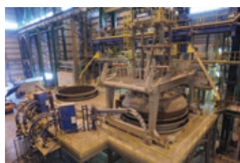
Figure 4: Interpipe VD station and hydrogen distribution after vacuum for wheel steel
