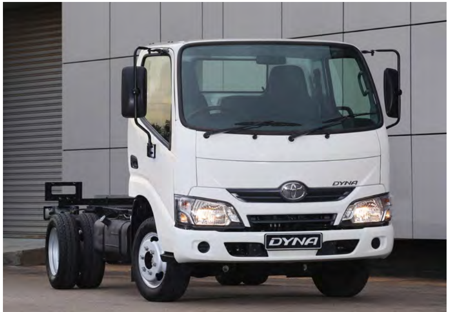
The vehicle now has a GVM of 3 500 kg, which means it is now classified as an LCV.
