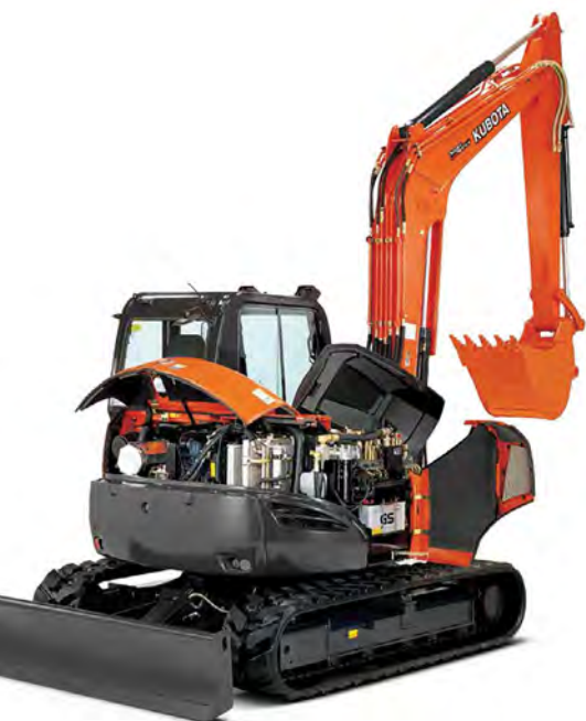
The KX080-3S's triple-opening bonnet offers greater ease of serviceability.
