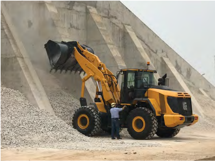
The key innovations of LiuGong's new Vertical Lift wheel loader are the vertical lift loader arms on an articulating frame and the mechanical self-levelling Z-bar bucket linkage on a vertical lift loader – both said to be industry firsts.
