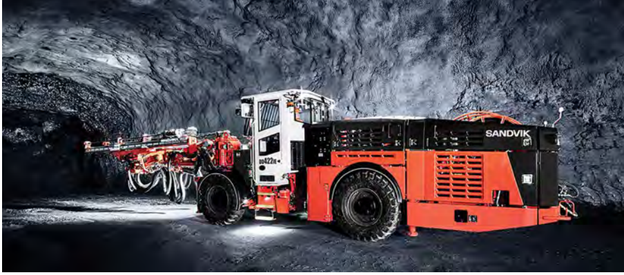
Sandvik's new intelligent rigs, such as the DD422i development jumbo, will soon include long hole drills and bolters.
