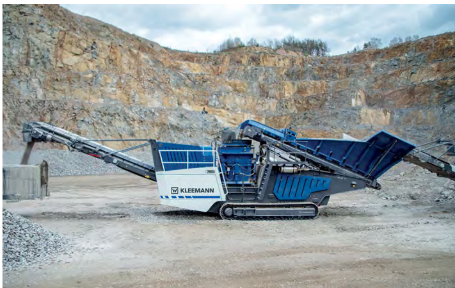
Designed for tough and demanding quarry applications, the cone crusher is powered by a diesel-electric drive and achieves an output of up to 470 t per hour.
