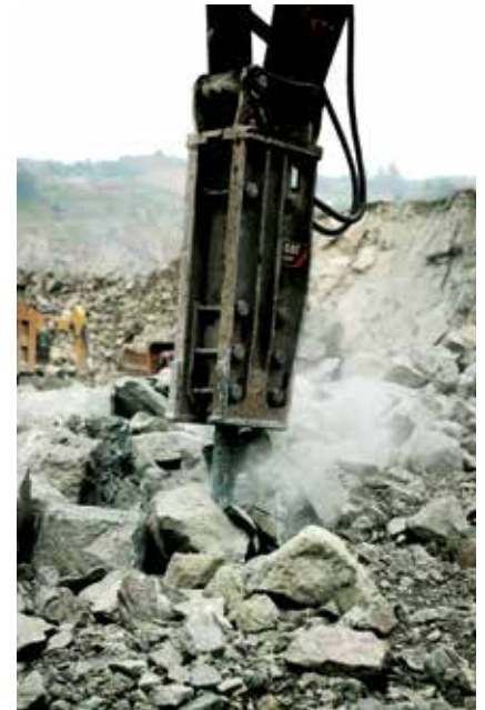
The top-mount (rectangular) style increases impact power by keeping hammer and stick forces in line.
