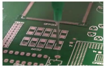
Even complex program patterns can be developed quickly using the simple point to point teach pendant. Dispense adhesive direct from syringes or optional metering valves and pressure pots. With fast indexing speeds, high accuracy and simple programming; robots are an ideal solution for most dispensing applications in a 400mm x 400mm work area. CE approved. Advanced features include work pattern array copy, end of cycle brush or wipe mode and slope dispensing.
