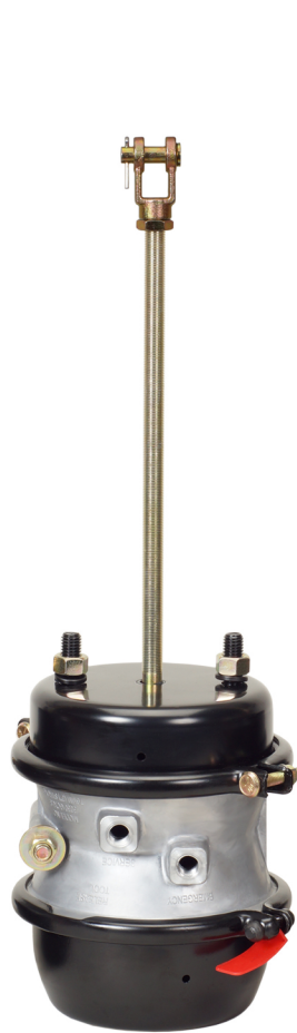
Part No. 3030CLE Long Stroke 14" Pushrod Length Square Ports
