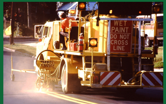
The City's old paint truck left the operator exposed to the elements.
