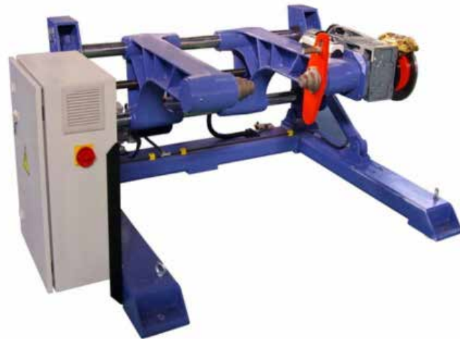
▲ The new 1,250mm take-up and tension payoff
