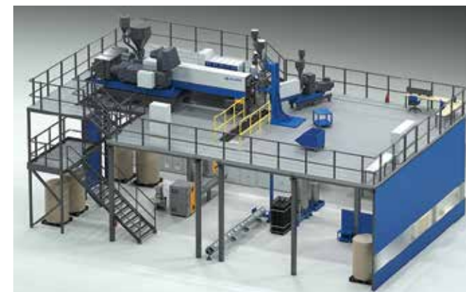
▲ A pilot-scale vertical extrusion group for medium and high voltage cable production in Mailefer's R&D center in Finland
