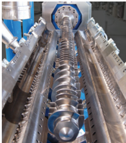
▲ The continuous kneaders from X-Compound have a wide range of applications – including gentle processing of cable compounds
