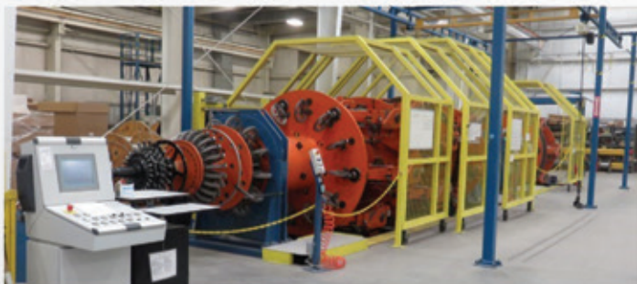
630mm Cortinovis Planetary Line 6+18
