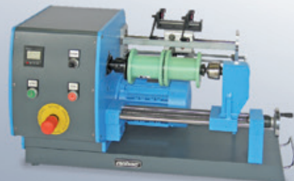
Spooler for spools Ø 60 - 200 mm, available with one or two spool seats, with revolution counter to preset and automatic stop, with spool take up via adjustable pinde and follower tip available with mechanical or laser sensor controlled traverse unit
