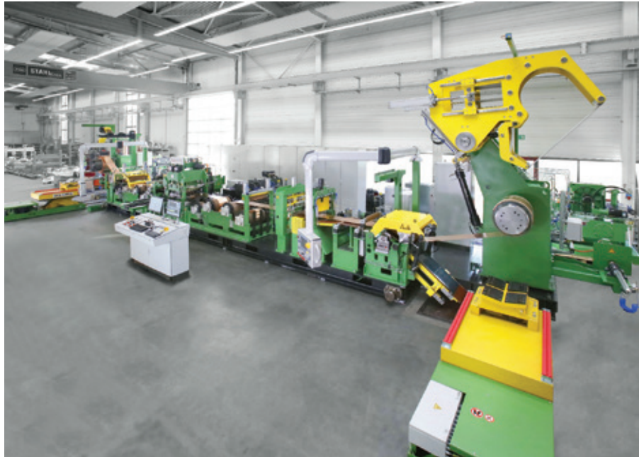
▲ A feed-in system without a manual feeder, developed by B+S, contributes to ease of operation and the economic efficiency of the line. The beginning of the strip is clamped in a clamping bar at the beginning of the line and pulled through to the outfeed. This means that no pilot strip is required, and welding or the need for guide plates is eliminated. Winding on the recoiler also takes place automatically
