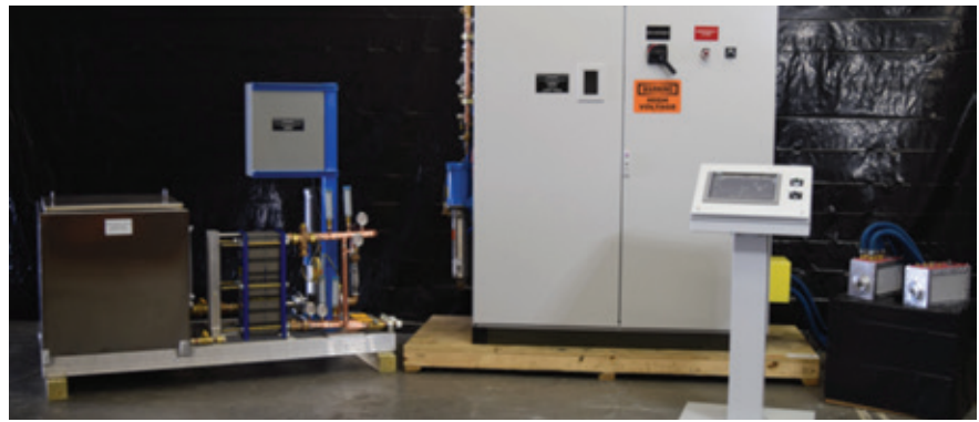
▲ MHD Power Supply, coils and cooling system
