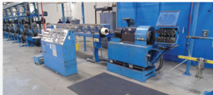
Tensor SZ Cabling Line
