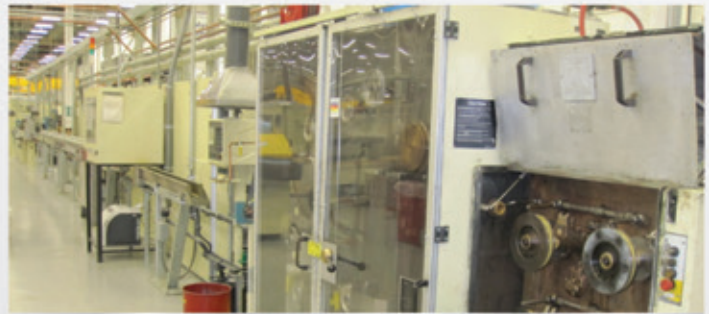
60mm Nokia/Niehoff Tandem Wire Insulating Line
