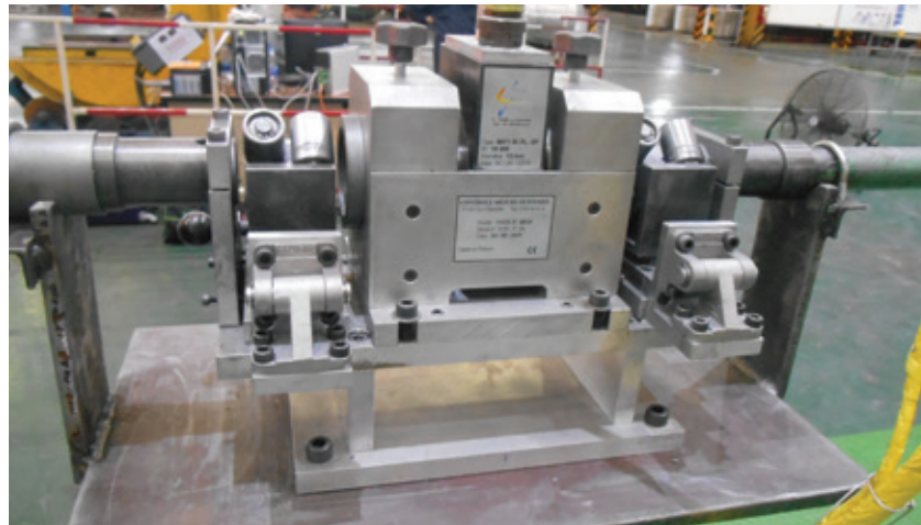
▲ The eddy current system from CMS
