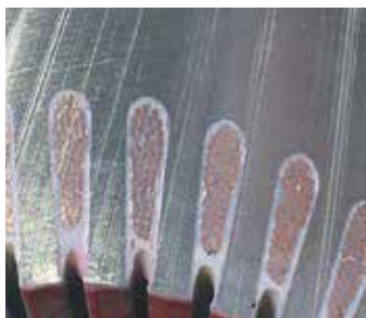
Figure 1: Secondary resin insulation holding coils together [6].
