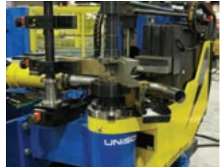
Unison has engineered a combined tube bender and cutter with a programmable all-electric architecture
