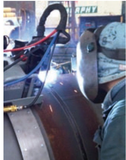
Gullco's Pipe Kat is mounted on the pipe using a quick mount pipe band
