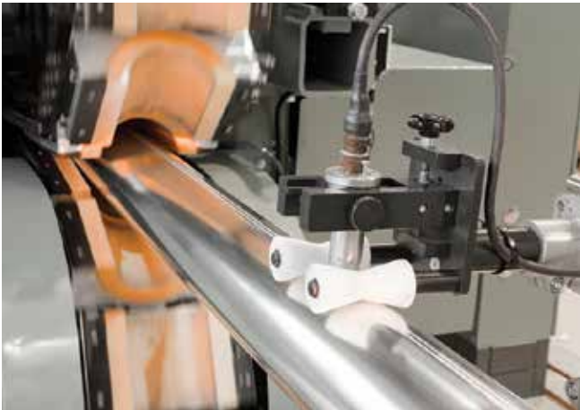
▲ Rosendahl RH-W metal tape forming and welding line for HV power cables
