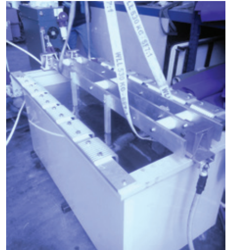
The mini-plant for testing the new pickling process without the use of hydrofluoric acid
