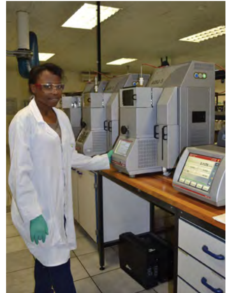
WearCheck's senior lab technician Lizzy Chabangu operates the new ADU5 distillation unit.
