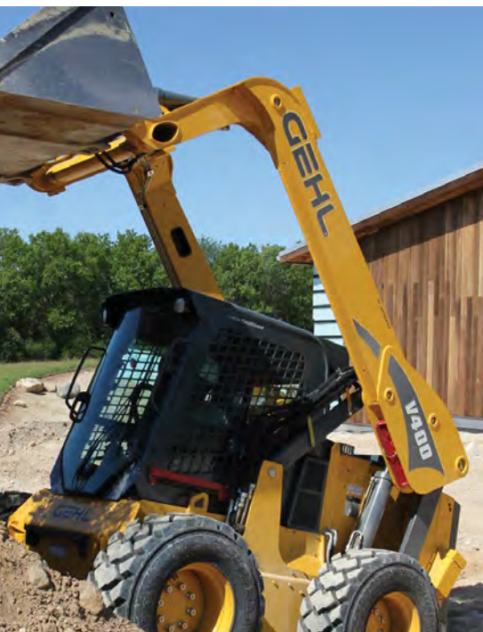
A compact loader scores on a variety of features, namely longer wheelbase, longer reach, better fuel consumption, better tyre wear, as well as ease of maintenance as accessibility to service points is generally better.
