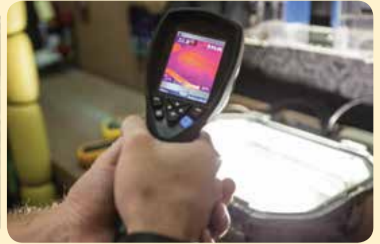
Thermal analysis of a luminaire using an infra-red camera imaging to measure temperature and record heat gradient/transfer for assessing thermal management properties.
