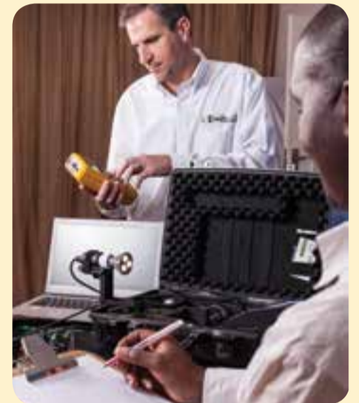
Energywise lab technicians, Daniel Zuczek and Nathi Msweli, using a power analyser and mini-goniometer to measure and record photometric and electrical performance of a light source.
