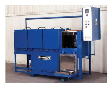
The oven features 4 inch thick insulated walls, aluminized steel exterior, type 430 stainless steel interior, four independently hinged doors to expose the front and back of each loading station, a steel plate oven floor and a workspace floor reinforced for 100lb loading on 1/4 inch plate.
