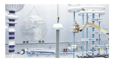
The company believes it has developed the world's first circuit breaker for high voltage direct current (HVDC). A combination of fast mechanics and power electronics, it will be capable of interrupting, within 5 milliseconds, power flows equivalent to the output of a large power station.
