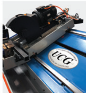
U-Saw high-speed flying cold saw
