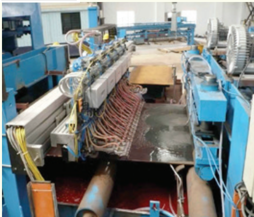
Spiral mill 2 m coil - Thickness 5 - 25 mm
