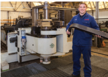
The powerful Elect 130 is capable of bending round tube up to 130mm diameter and the equivalent square or rectangular sections
