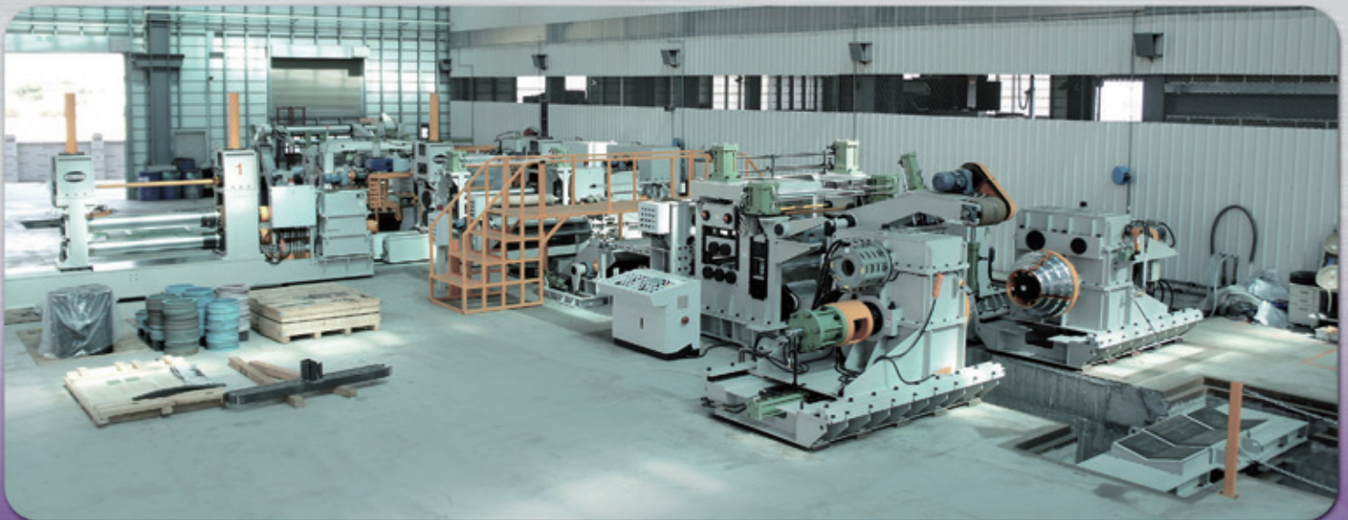
● 27 Tons 1600mm x 8t slitter
