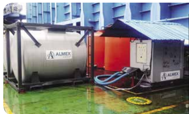
Dust Suppression System
