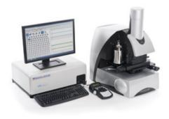
The Morphologi G3-ID brings a significant additional capability to the Morphologi range of instruments – the ability to provide chemical identification of individual particles using Raman spectroscopy.
