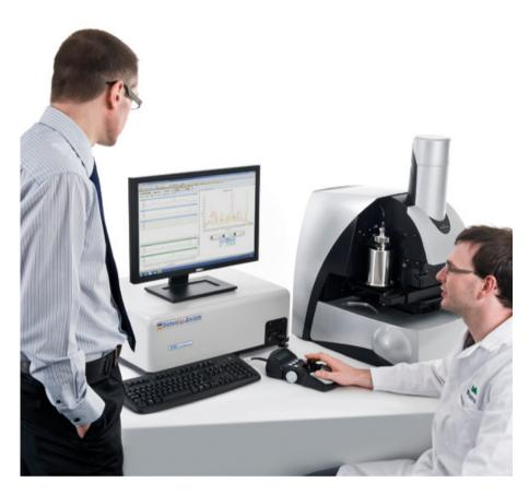
The Morphologi G3-ID provides a unique capability, combining automated static imaging features of the Morphologi G3 with chemical identification of individual particles using Raman spectroscopy. This fully automated instrument is designed to allow both particle characterization scientists with limited spectroscopy experience and more experienced spectroscopists to get an in-depth understanding of their particulate samples.
