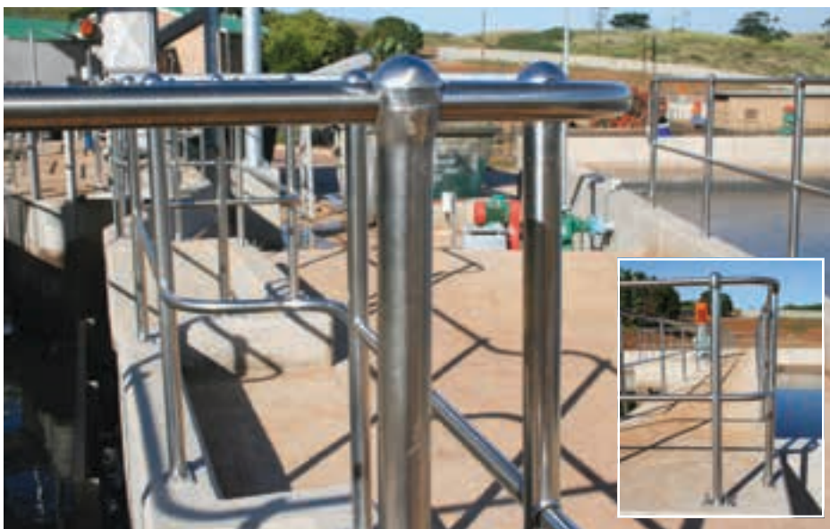
Stanchions on the Andrew Mentis stainless steel handrails are 45 mm in diameter with a 2.0 mm wall thickness and the 8.0 mm thick base plates are designed to allow moisture to drain from the stanchion. Inset: Stainless steel handrailing offers numerous benefits, including increased safety and hygiene.
