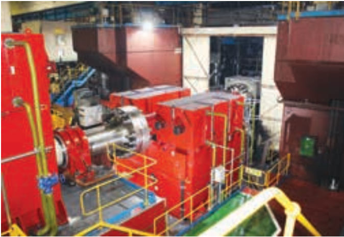
Left: Two of Europe's largest synchronous motors ever used in a reversing roughing mill have been commissioned by ABB at Tata Steel's Port Talbot hot strip mill in South Wales. Right: The upgrade aims to increase steel production significantly while improving final product quality.
