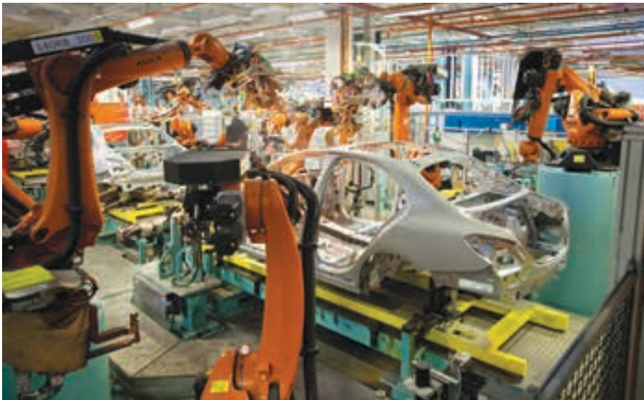
The cutting-edge production technologies linked to the new C-Class include components and processes such as aluminium skin panels, complex laser welding, roll forming for complex structural profiles, advanced rear axle carriage assemblies, aluminium pre-treatment and natural fibre pressings.
