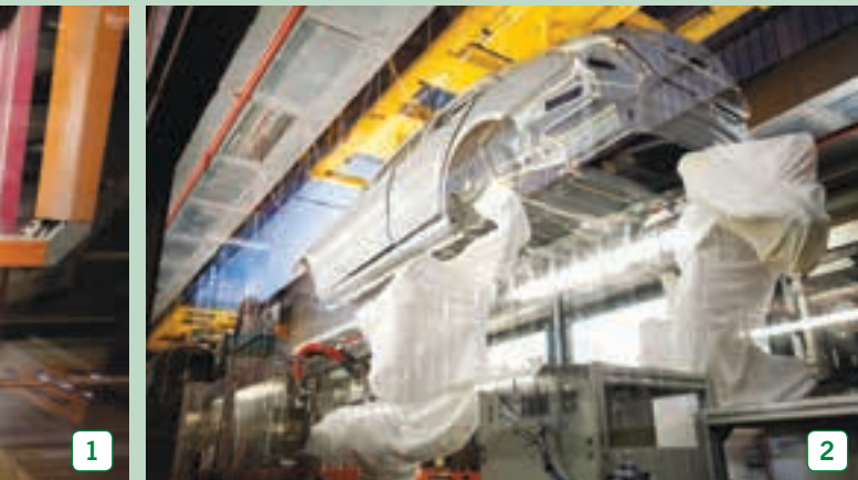
1. A vehicle enters a chemical dip tank during pre-treatment. The entire body is submerged so that all crevices can receive chemical treatment. 2. Protected robots seal the underside of the body before painting. 3. A pre-treated vehicle enters the painting line. Each vehicle receives three coats of paint, starting with an inspection stage where any visible defects are removed.
