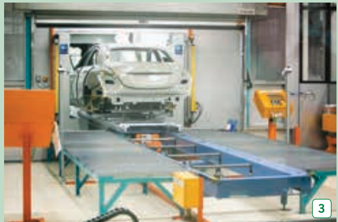
1. A vehicle enters a chemical dip tank during pre-treatment. The entire body is submerged so that all crevices can receive chemical treatment. 2. Protected robots seal the underside of the body before painting. 3. A pre-treated vehicle enters the painting line. Each vehicle receives three coats of paint, starting with an inspection stage where any visible defects are removed.
