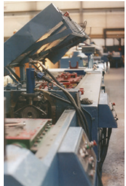
▲ Transducer/die assembly fitted to a Schumag drawing machine
