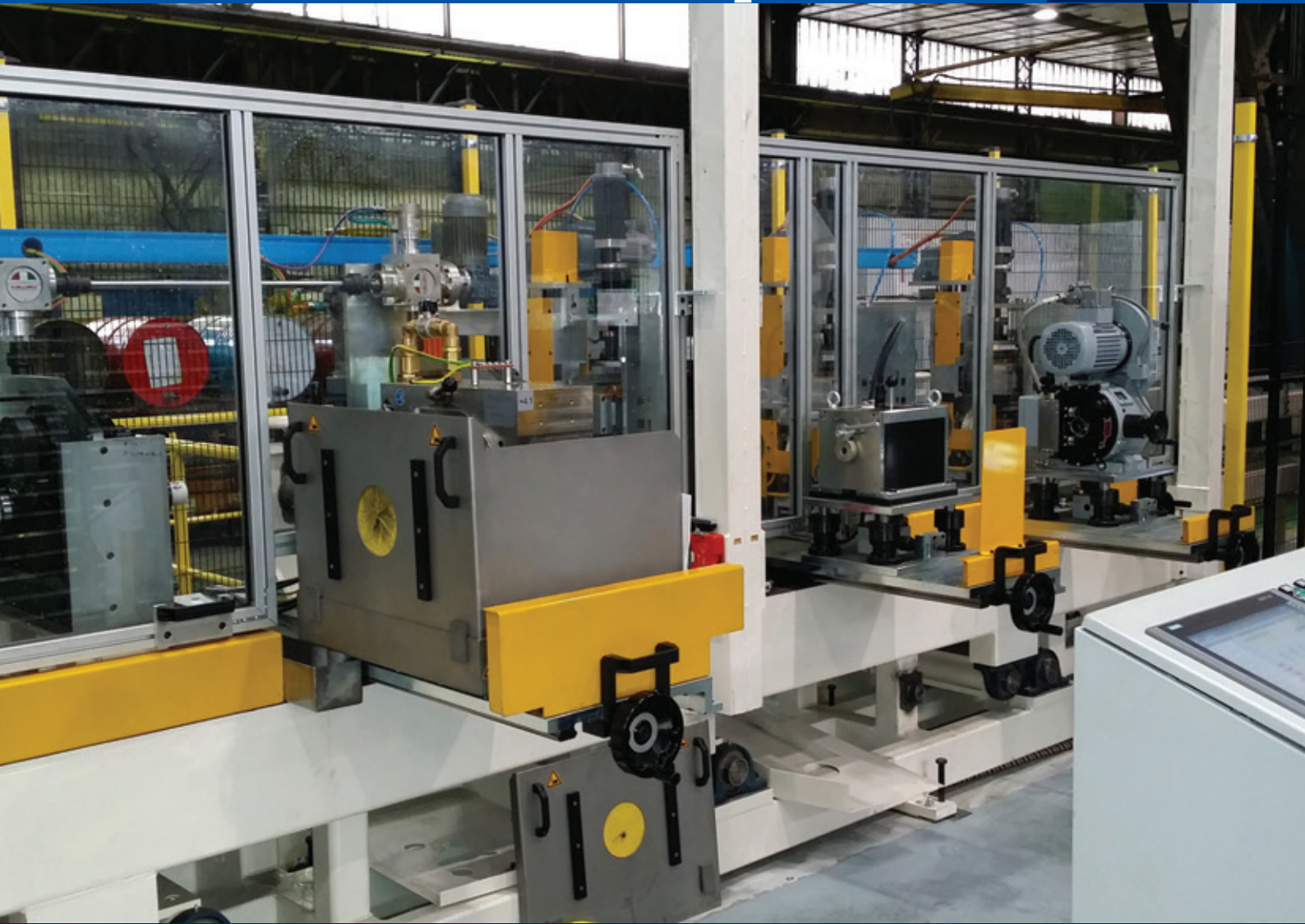
▲ Ugitech has invested almost €2m in a new ultrasonic test unit at its production site in Ugine and has thereby increased its capacity in quality assurance for steel bar
