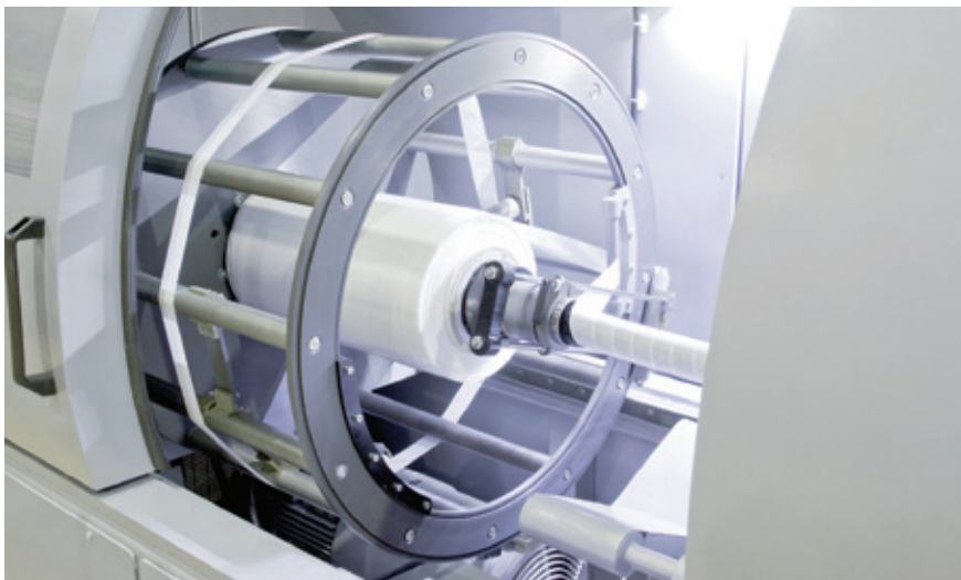
▲ Rosendahl's helical tape applicator Rota 500
