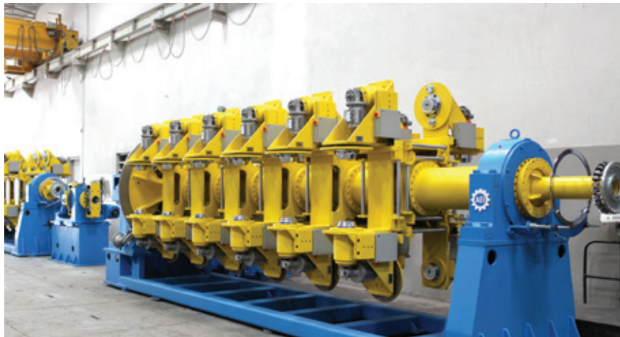
▲ Rigid stranding machine from AEI Machines
