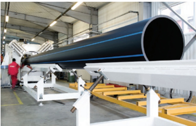
A 1.2m pipe with colour stripes produced on the battenfeld-cincinnati line (Photo credit: © TehnoWorld)
