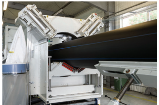
The cutStream PTA 1200 cutting tool can cut both swarfless or with swarfs, depending on the application (Photo credit: © TehnoWorld)
