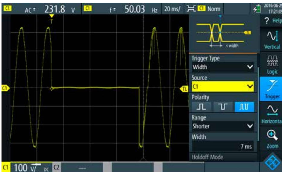
Fig. 4: Powerful trigger functions make it possible to specifically detect power quality problems. Brief power supply interruptions due to poor contacts are quickly detected with the pulse width trigger. Source: Rohde & Schwarz
