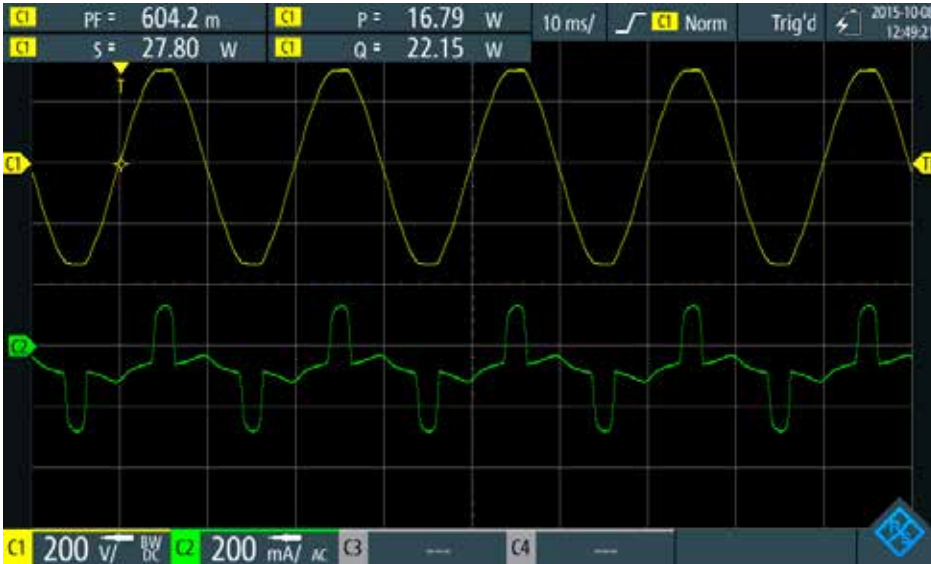
Fig. 5: Automatic measurement functions calculate apparent, active and reactive power as well as the power factor from the measured voltage (channel 1) and current (channel 2). Source: Rohde & Schwarz
