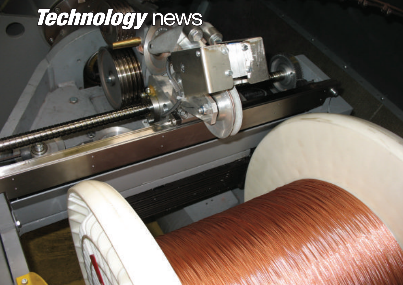
○ The new NBAT automatic opto-electronic traversing system for Niehoff bunching machines
