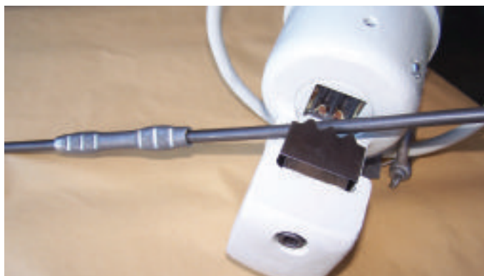
○ Petig's Hydrocut used to join wire ends by crimping
