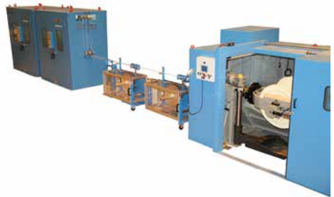
▲ Setic backtwist pairing/quadding, 800mm
