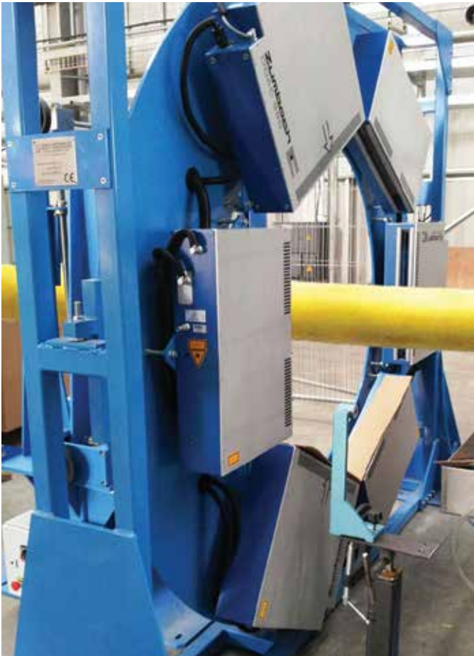
▲ 3-axis ODAC 550 system, measuring an offshore cable of 500mm OD
