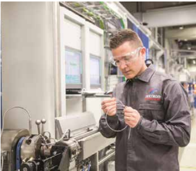
▲ Rosendahl extrusion line for high temperature materials
