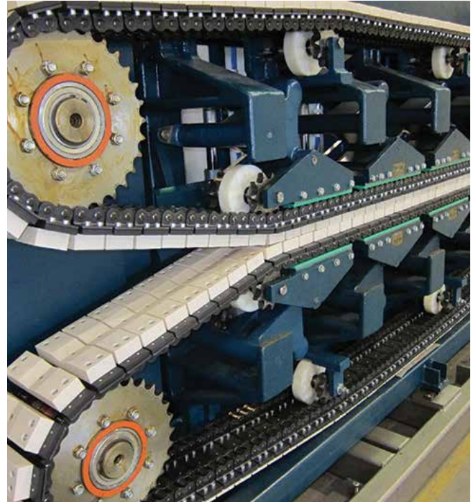
▲ The chain-type capstan with two-ton pull from Queins
