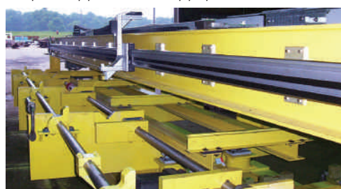
Figure 2: This system is capable of processing pipe from 1.90" OD to 5" OD, handling lengths from 15-48ft, with a max weight of 1,500lbs. The Compact WMS shown can process pipe at a rate of 5 pipe per minute
