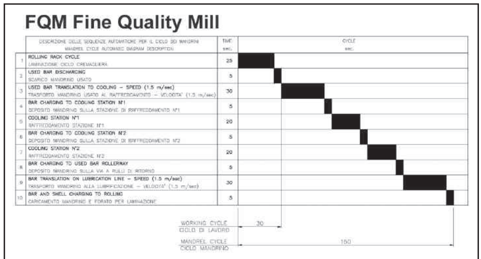
Figure 11 (above left): Into the heart of the FQM process; Figure 12 (above right): a diagram displaying the FQM's automatic mandrel cycle
