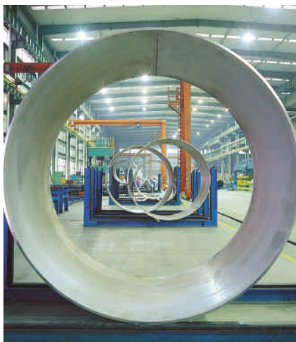
Jiuli manufactures seamless tube from 6-273mm OD and welded from 9.53mm to 2,540mm OD
