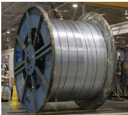
i A reel with 30,000ft of RathGibson zinc clad, lean duplex subsea umbilical tubing destined for installation off the west coast of Africa
