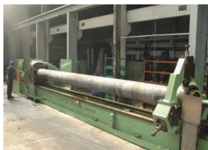
i The boring of 475mm x 9m thick walled tubes used for the international energy market
