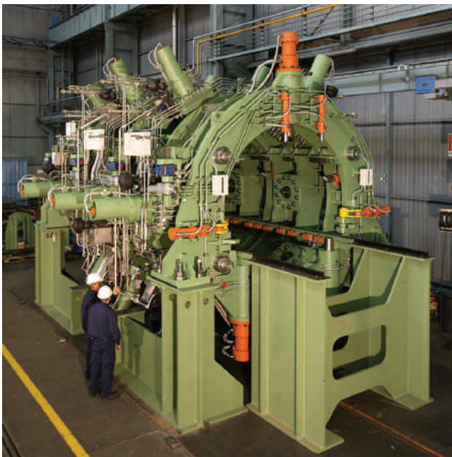
Figure 13: A complete view of a five-stand FQM™ (Fine Quality Mill) for a 350,000t/y 7" seamless pipe mill (Buttrio, Italy)
