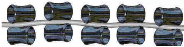
ⓘ Roll configuration: the 10 roll machine
