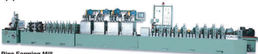
Pipe Forming Mill Pipe O.D Range 1/2"~24"
