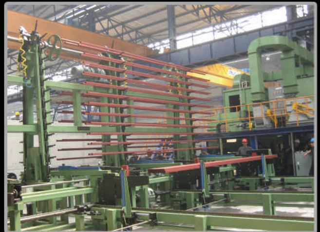
Factory space save by tube dry elevator
