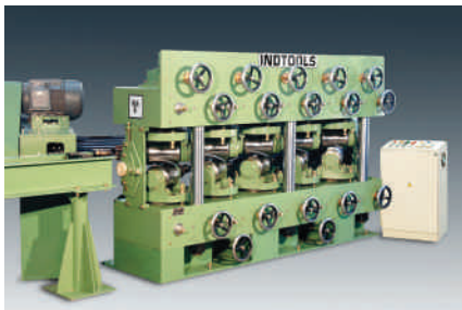
ITL's straightening machines are supplied with 6, 10 (above) and 14 rolls
