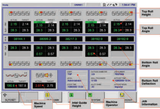
Computer setting systems ensure more accurate roll positioning
