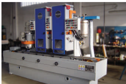
① Model RSP 400/3000/2U-200 + orbital brushing unit is ideal for making deburring operations on blanked pieces
