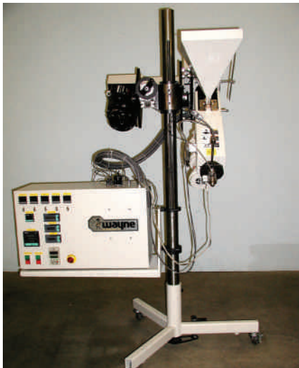
Wayne Machine's new vertical extruder series features balanced weight distribution
