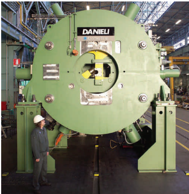
Figure 3: The 3-roll FQM mill (above) provides a more uniform deformation in the pass than was previously experienced with the 2-roll RMM process
