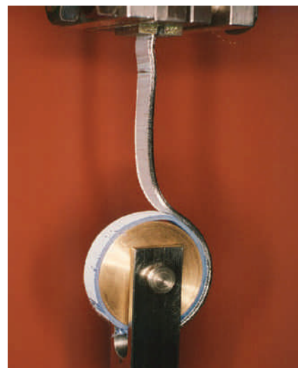
Aluminium layer peeled off plastic medium pipe
