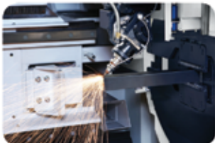
3D laser cutting of complex or angled configurations of long pipe and structural materials
