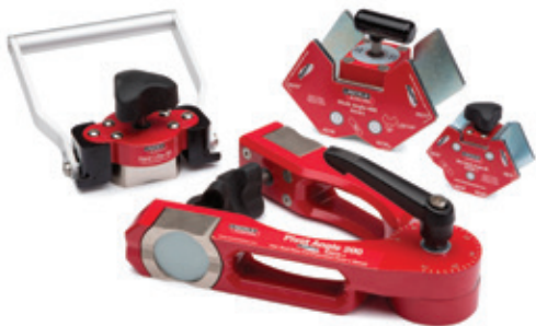
Lincoln Electric magnetic fixturing tools can be used to position steel for tacking or lifting sheet steel at the work table
