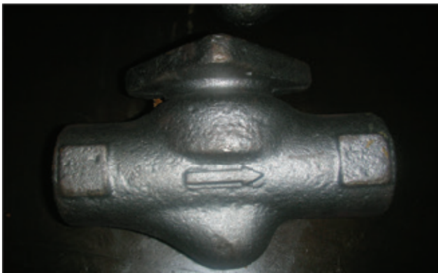
Stem with low section thickness, susceptible to quench cracking.
