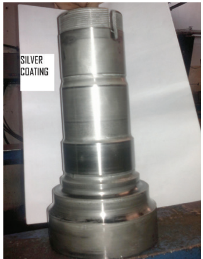
Image 2: Fully machined spindle re-heat treated by applying anti-scale compound. Zero scaling observed. Aesthetic appeal is intact
