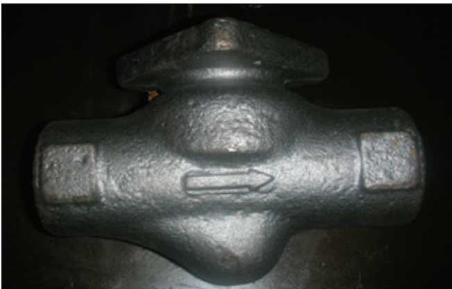
Image 5: Coated with ESPON anti-scale compound before re-heating. No scale pit marks
