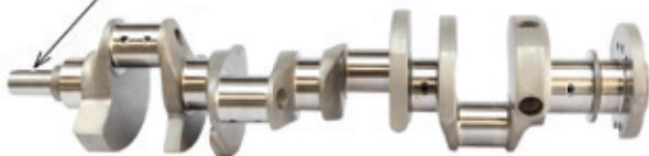
Stem with low section thickness, susceptible to quench cracking.
