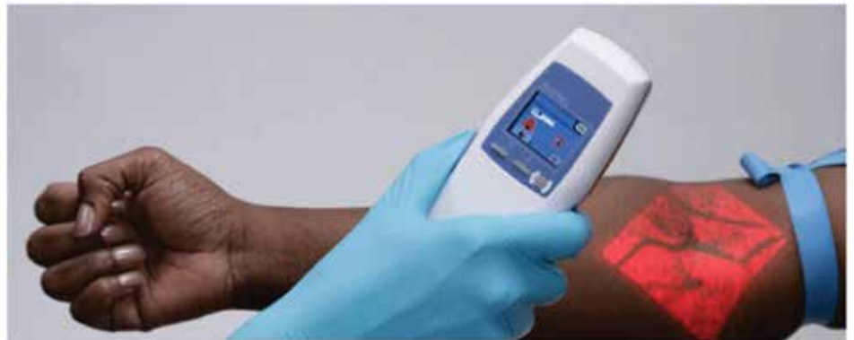
Figure 1: The rechargeable AV400 AR scanner weighs less than 10 ounces and displays the veins underneath the skin. (Image source: AccuVein)
