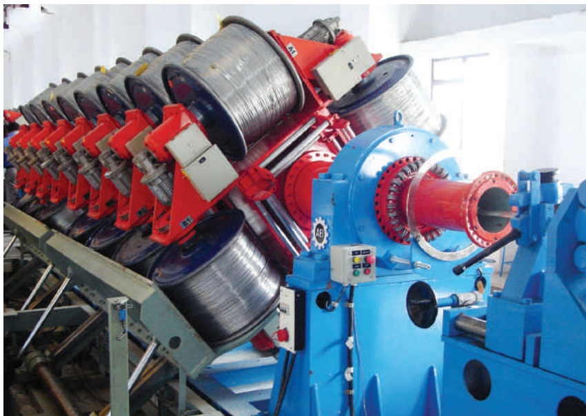
○ The new strander weighing in at 140 tons
