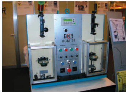
○ HGM-21 – High speed wire-type ND/PCD die sizing/polishing machine
