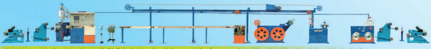
Ø70 data cable (cat. 5, ultra 5, 6) PLC jacketing line (also used for framework cabling & 4-25 pairs data cable jacket)
