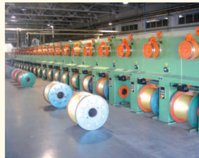
○ Spool take-up frame with double accumulation capstan for non-stop operation
