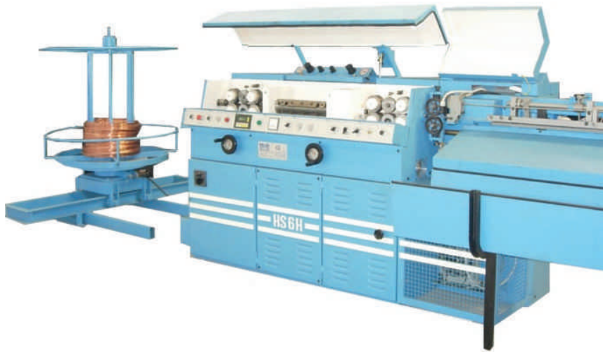
Delisi's Model HS6H with hydraulic and flying shear cut for wires from 1.5mm to 6mm features four pairs of feeding rolls and rapid change of diameter
