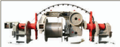
○ The new double twist strander model CDT-2000 from CM Caballe
