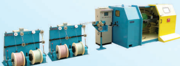
HD- \phi 800 PLC 4-pairs twisting cabling (optional framework cabling)
