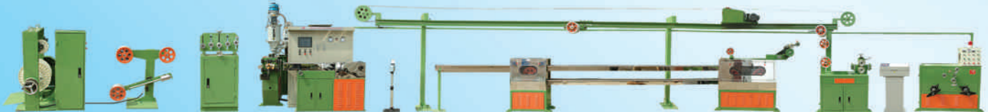
Ø30, Ø45, Ø65, Ø90 PLC control, PTFE (Hi-temperature) extruder
