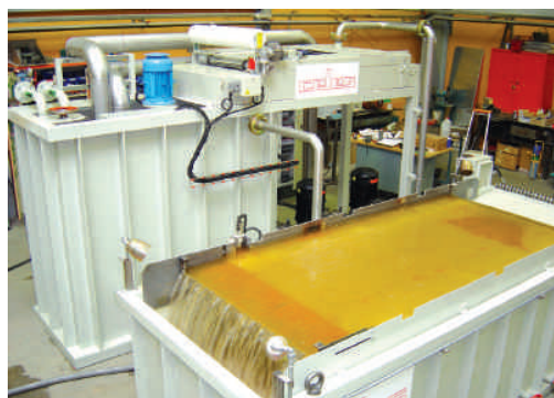
○ Oil quenching of threads from Celes
