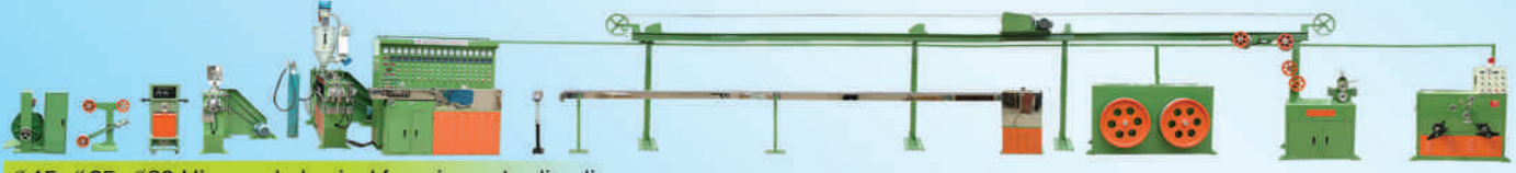
Ø45, Ø65, Ø90 Hi-speed physical foaming extruding line
