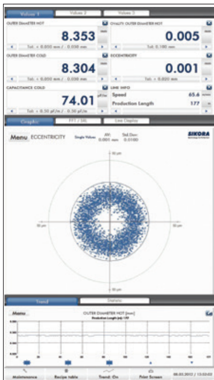
○ Picture 4: Ring type distribution of the single values of the eccentricity
