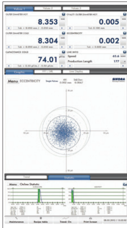
○ Picture 3: Random type distribution of the single values of the eccentricity
