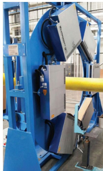
○ 3-axis ODAC 550 system, measuring an offshore cable of 500mm OD
