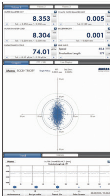
○ Picture 5: Ellipse type distribution of the single values of the eccentricity
