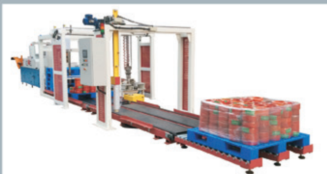
Auto coiling and stacking line
