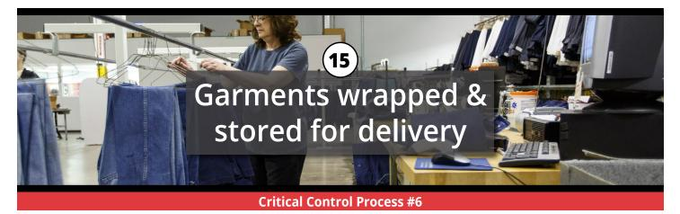
Final inspection on the clean garments is performed by the operator per the Corporate- Garment Quality Specifications. The clean garments are wrapped appropriately to minimize cross-contamination and are now ready for delivery back to the customer site.
