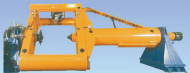
DJ01400-02500B Single twisting machine
