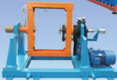
DJ0630-02500A Single twisting machine
