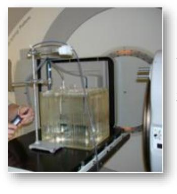
**Beam output measurement** at the energy used for the trial in the institution reference condition
