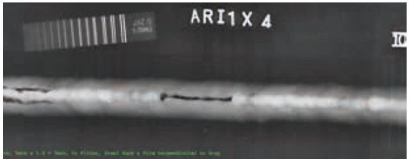
A digital radiograph of a 12 mm plate weld with an SNR of 111.3 measured in the parent material. This meets the SNR minimum requirements of 98 (1.4 times 70) if not measured in weld the weld metal.
