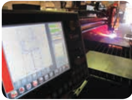
Koike's Katana-ADV CNC controllers incorporate all of the software for controlling the cutting path of the torches, along with the electrical, flame and gas controls for the cutting process being employed.
