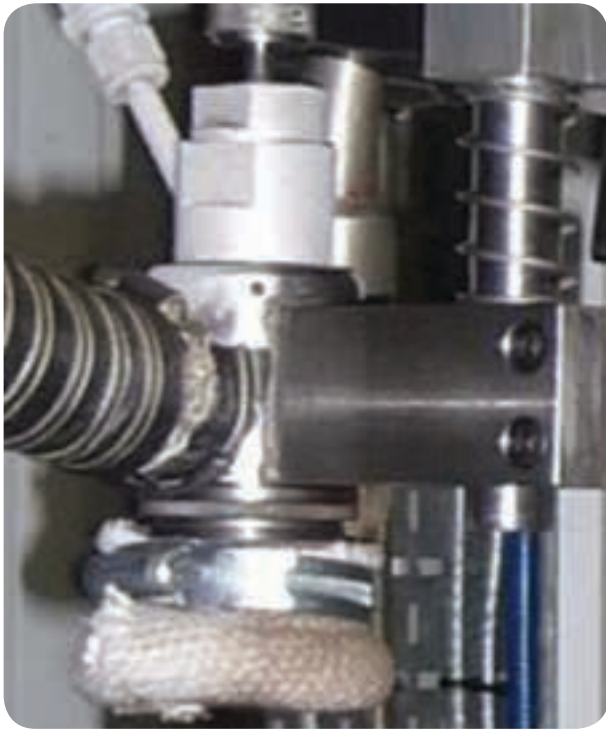
Figure 2: Close-up of the cooling delivery head with coolant seal in place, and through head extraction.
