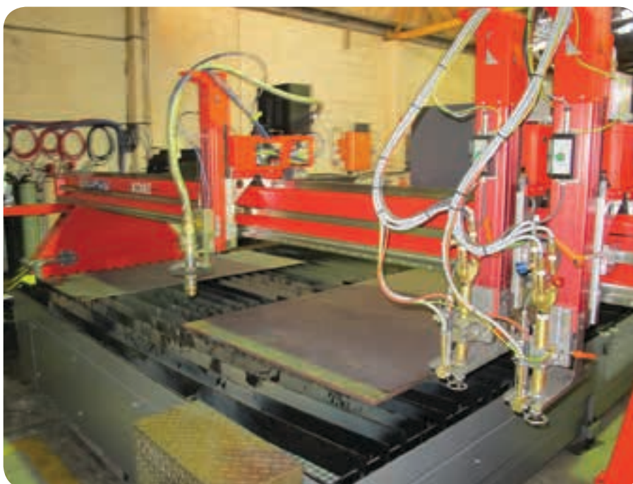
The Koike Deltatec 4500 CNC cutting system chosen by Laser Junction. The machine has an effective cutting area of 3x12 m; a Hypertherm HPR260XD auto gas control, high-definition plasma cutting system; and two fully automated Koike K-FIT oxy-fuel cutting torches.
