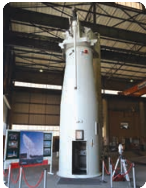
Efficient Engineering's current flagship project is for the Meerkat antennas for the Square Kilometre Array project (SKA). The company is completing the fabrication and full electrical and mechanical integration of the yokes and pedestals for the first 64 Meerkat antennas.
