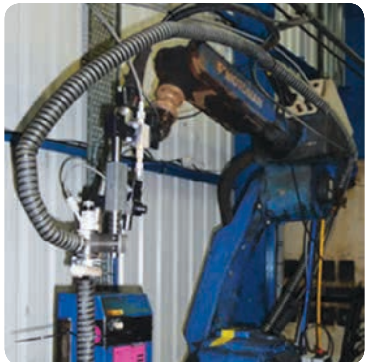
Figure 1: The LSND welding system mounted on a robot in the industrial trial facility.
