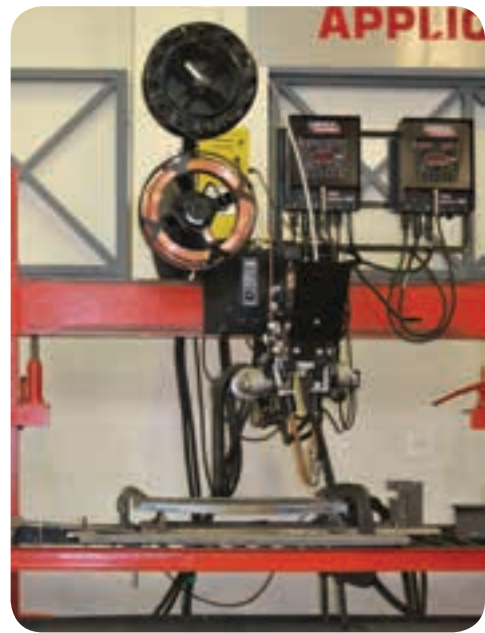
Lincoln Electric's WTC in Midrand is promoting next-step welding technologies such as Tandem submerged-arc welding with Lincoln PowerWave ac/dc power sources.
