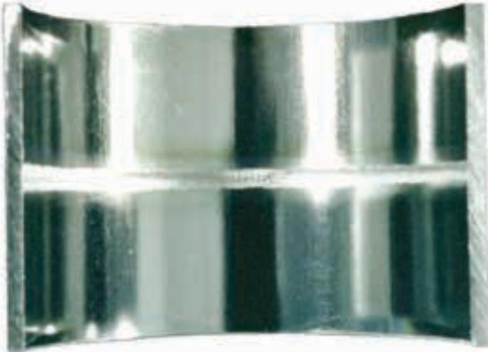
Figure 1. An example of an ideal weld, a TIG orbital weld on 316L electro-polished stainless steel pipe.
