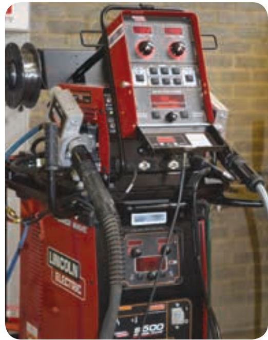
Above: A Bug-O Piper Plus mechanised welding systems ready for use. These systems are commonly used with Outershield 91K2-HSR flux-cored welding wire for fill and cap passes. Right: Lincoln Electric's Power Wave S500 with the addition of an STT® Module has the fast digital communication necessary for controlling the root welding process for consistent penetration and bead profile.
