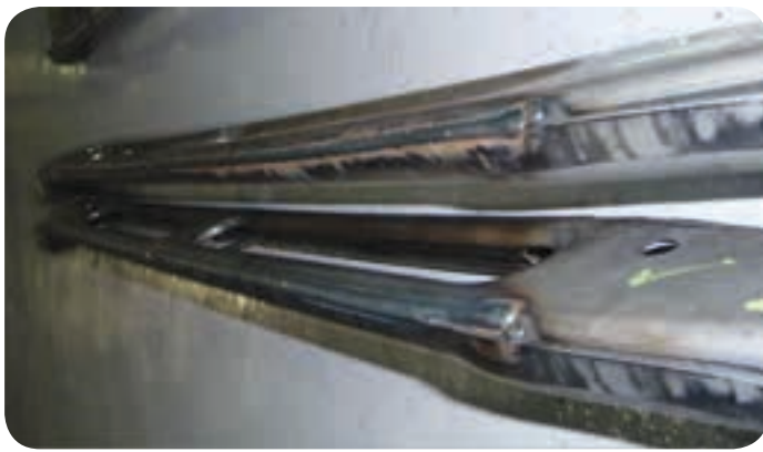
Figure 15: A comparison of the effect of distortion on repeatability and weld quality on typical LSND (top) and conventional GMAW welded (bottom) beam parts manufactured in the trial. It can be seen that the induced distortion in the conventionally welded part causes the weld path to drift off the seam.
