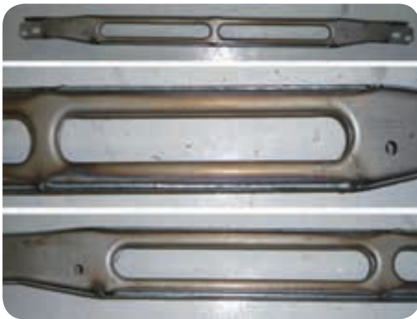
Figure 13: Images of the trial bumper beam sub-assembly showing the weld pattern used for the trials.
