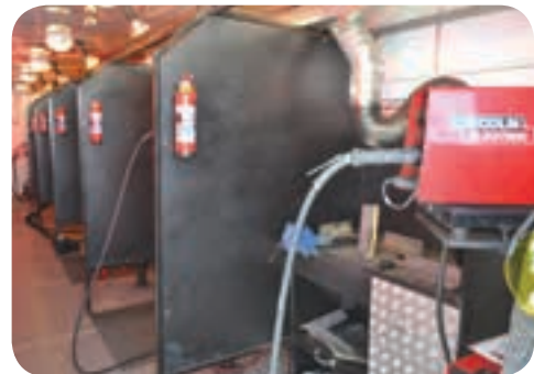
The company has developed a containerised welder training centre for on-site approvals, welder testing and training.
