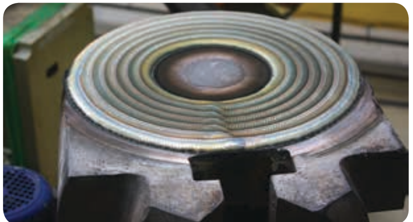
A PTA-applied hardfacing coating on a high temperature steam valve components.
