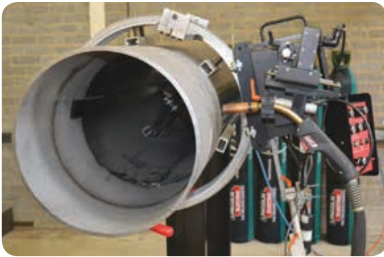
Above: A Bug-O Piper Plus mechanised welding systems ready for use. These systems are commonly used with Outershield 91K2-HSR flux-cored welding wire for fill and cap passes. Right: Lincoln Electric's Power Wave S500 with the addition of an STT® Module has the fast digital communication necessary for controlling the root welding process for consistent penetration and bead profile.
