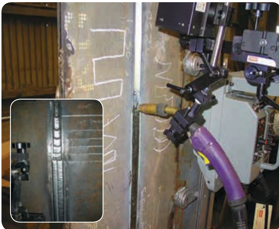
Mechanised flux-cored wire welding with the UTP AF 6222 Mo PW wire and (left) a typical high quality joint.
