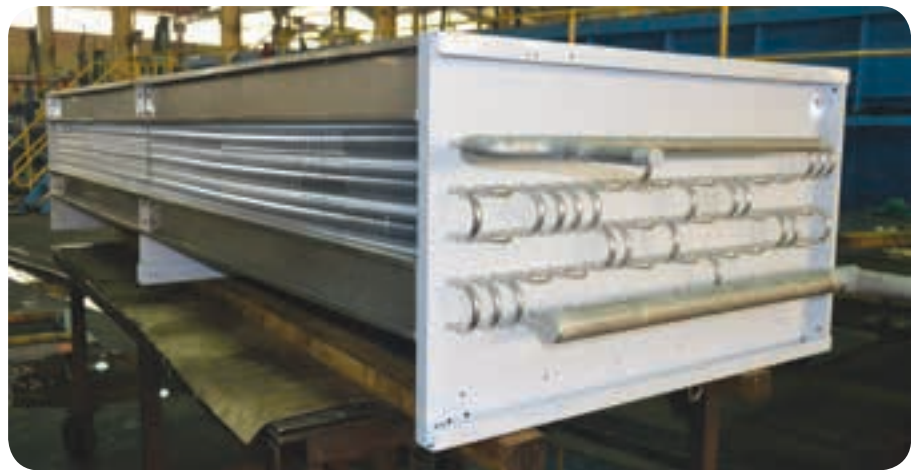
Above: The welding of HCHE's heat exchangers involves significant amounts of stainless steel: 304 and 430 grades on tubes, pipe and plate.
