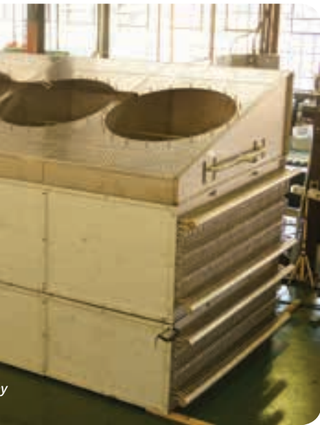
Above: The welding of HCHE's heat exchangers involves significant amounts of stainless steel: 304 and 430 grades on tubes, pipe and plate.
