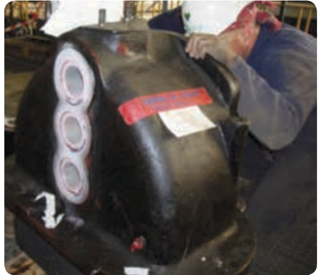
Particle testing (PT) on the piping inlets of an oil pump.
