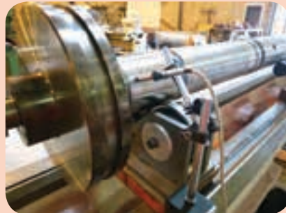
Burnishing is used to improve run-out measurement reliability, which can significantly improve the in-service condition-monitoring accuracy for rotating equipment.
