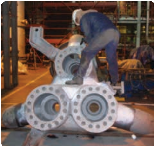
Ultrasonic testing (UT) taking place in a three flanged piping manifold.
