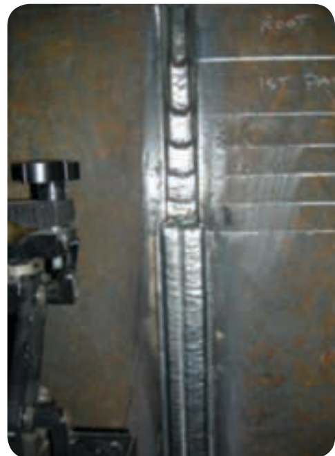
A test plate of the flux-cored wire UTP AF 6222 Mo-PW (AWS A5.34 ENiCrMo3 T1-4) welded in vertical-up position.
