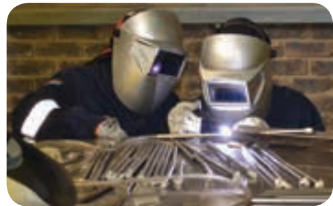
Right: TIG welder training taking place at HCHE's Elandsfontein premises. "Almost all of our welders are qualified for tube welding using TIG," says Banza.
