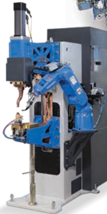
The nut-welding system can be attached to the right or left of the spot welding cell with a dedicated handling robot (MH5) attached to the side structure.
