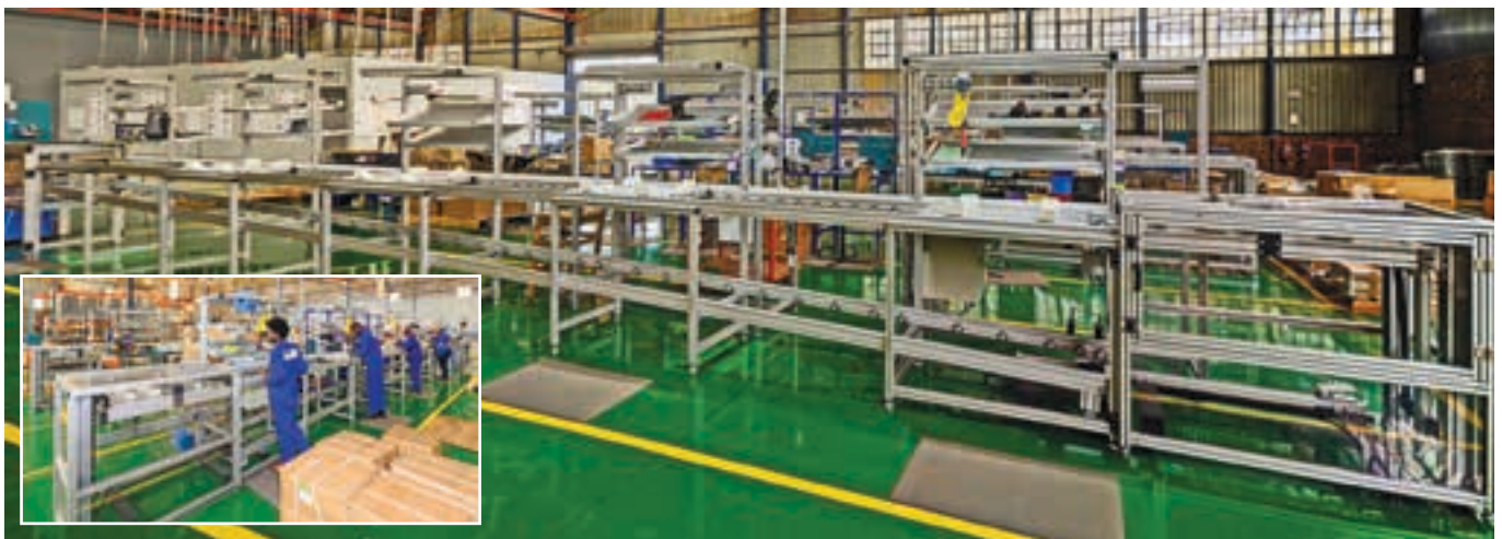
Side view showing the assembly line. The inclined level of the MPS is used to return the assembly trays to the first workstation following the delivery of a completed light to quality inspection at the end of the line. Inset: The 10 m MPS lanes each consist of five workstations, where operators assemble Beka Schröder’s LED luminaires on specialised aluminium trays.
