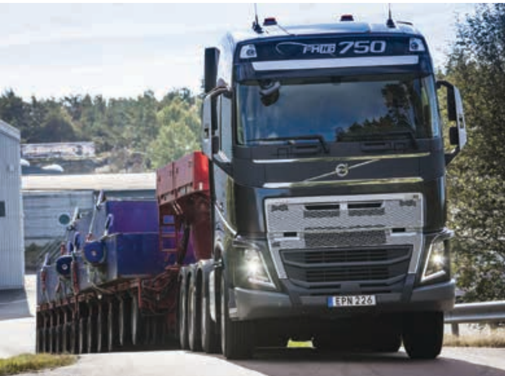
I-Shift makes it possible to add up to two new crawler gears, resulting, among other things, in the ability to start-off from standstill and transport a gross combination weight (GCW) of up to 325 t.
