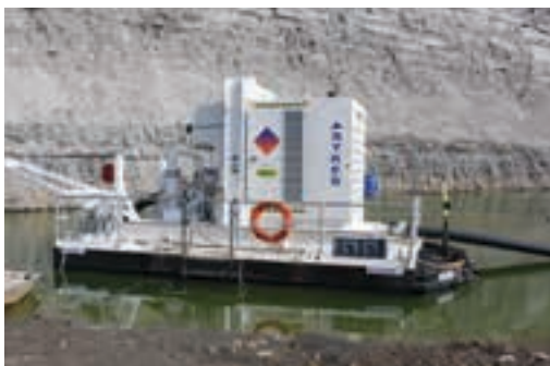
The Sykes extra high head (XH) pump range caters to the demands of the mining industry and all models have the ability to operate unattended at high discharge heads.
