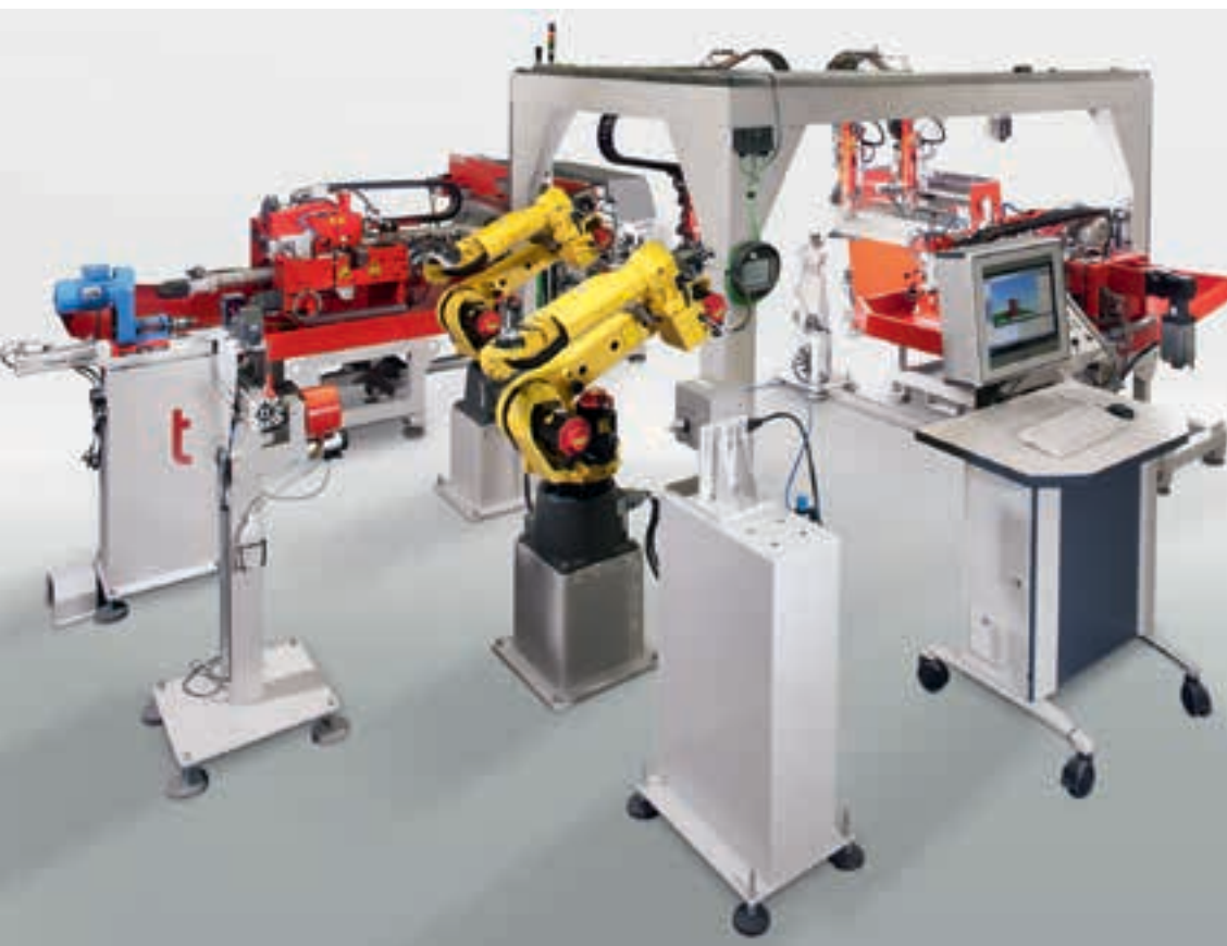
Complete production cells are specifically coordinated to meet tube production requirements. This includes the modification of the layout of interconnected modules to achieve the perfect material flow. Image® transfluid.
