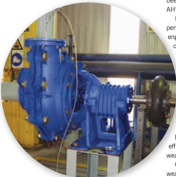
The Warman WBH slurry pump undergoing testing at the Alrode manufacturing centre.
