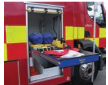
Featuring heavy-duty lock-in and lock-out mechanisms and a front latch release, Accuride telescopic slides are ideal for securing drawers in mobile applications.
