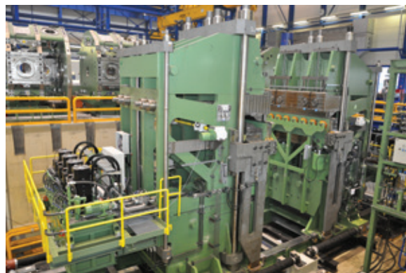
Use of the VSP drives in all pipe forming presses. Here: successful test run of the crimping press with VSP at the SMS Meer workshops in Monchengladbach, Germany
