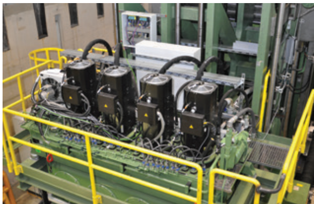
The gap closing press requires 50 per cent less energy than the older machine generations thanks to the variable speed pump control (VSP)
