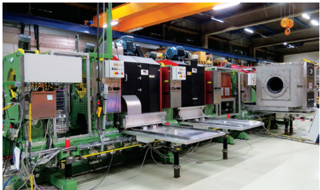
MAC's multi-test system for a Russian pipe mill. The Echomac 500mm Ultrasonic Rotary is shown on the far right, where it has been temporarily moved out for access during maintenance operations. The two black testers in the centre are the Rotoflux 500mm transverse and longitudinal units
