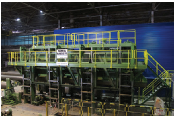
The gap closing press requires 50 per cent less energy than the older machine generations thanks to the variable speed pump control (VSP)
