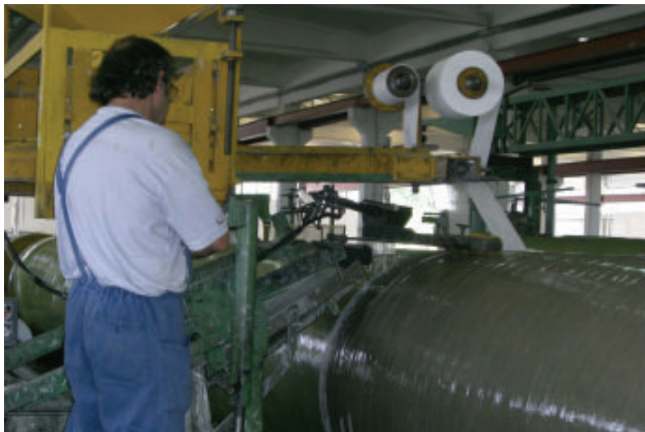
▲ Tailor-made fabrication: winding of an FRP pipe with diameter 1,000mm
