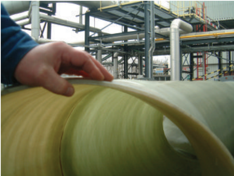
▲ Lightweight, fast assembly: cooling water pipe diameter 800mm
