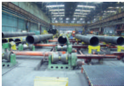
▲ US Steel Košice manufactures spiral-welded pipes from 406 to 1,420mm
