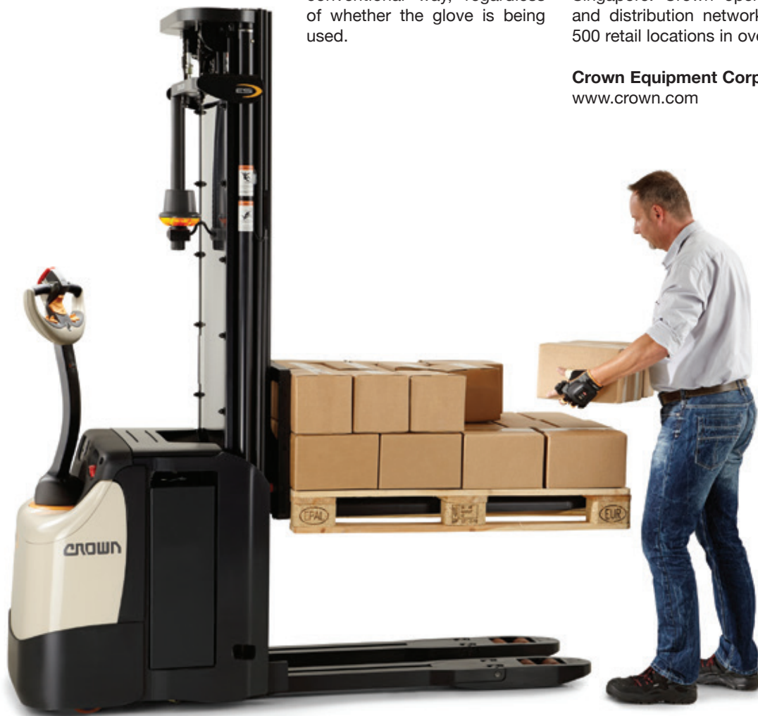
Crown's QuickPick Remote technology allows control of lift/lower functions via 'magic glove'
