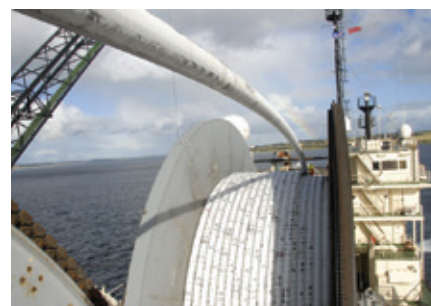
The pipe was designed to withstand the strains of the reeling process
