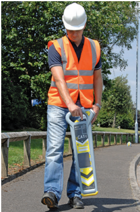
The gC.A.T4 in use, with a Genny4 signal generator on the path in the background
