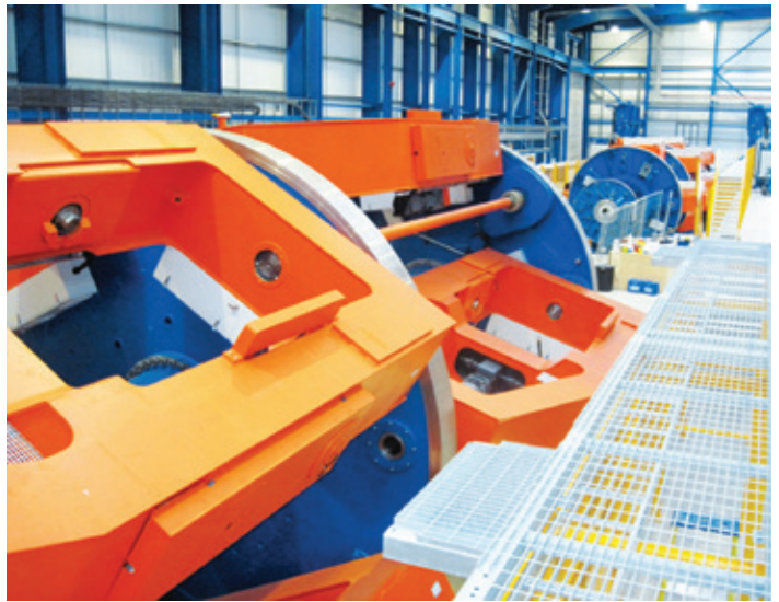
▲ Stranding machine type MKVS 1+16x2300+8x2700 delivered to Bridon in the UK
