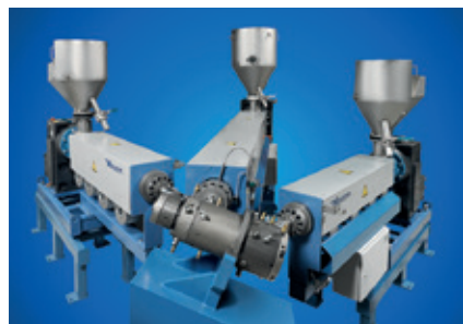
▲ Maillefer air-cooled triple extrusion group for CV lines
