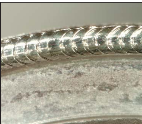
Laser Seam Weld of Pressure Cap
