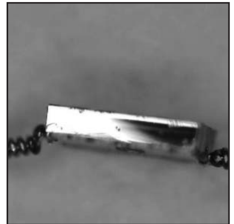
.003" Wire Welded to .003" Platinum
