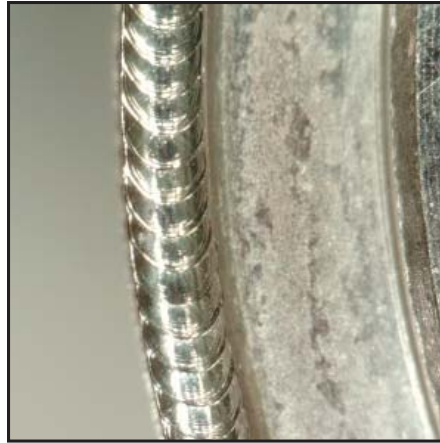
Laser Seam Weld of Pressure Cap
