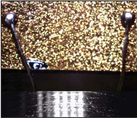
Laser Spot Weld for Solder Reflow
