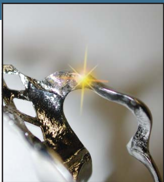
Laser Welded Clasp Repair
