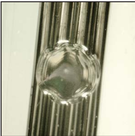
Laser Spot Weld of a Wire Bundle
