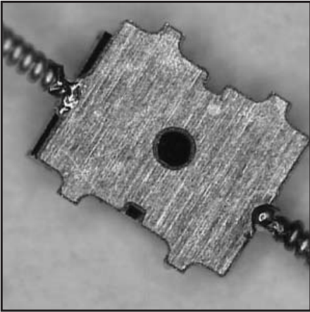
.003" Wire Welded to .003" Platinum
