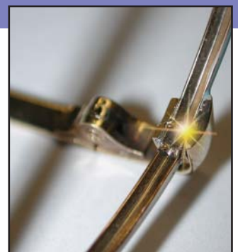
Frame Repair - Front to End Piece
