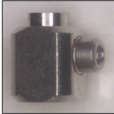
Set Screw Housing Structural Seam Weld
