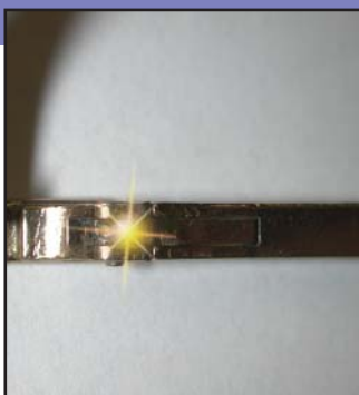
Hinge Repair Weld
