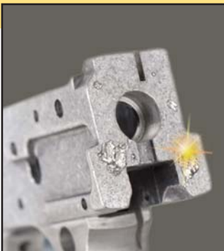
Titanium Casting Porosity Repair
