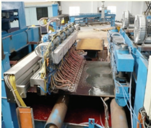
Spiral mill 2 m coil - Thickness 5 – 25 mm
