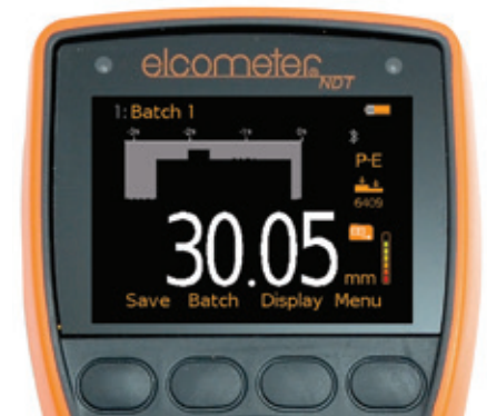
The top-of-the-range Elcometer MTG8 with ThruPaint™ Echo-Echo technology
