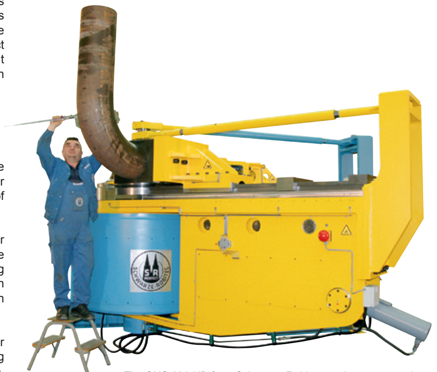
The CNC 320 HD from Schwarze-Robitec produces extremely small bending radii of 1.5 x tube diameter, even for very large, thin-walled tubes with a diameter of up to 323.9mm
