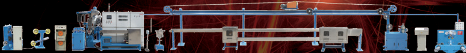
Wire and cable extruder line
