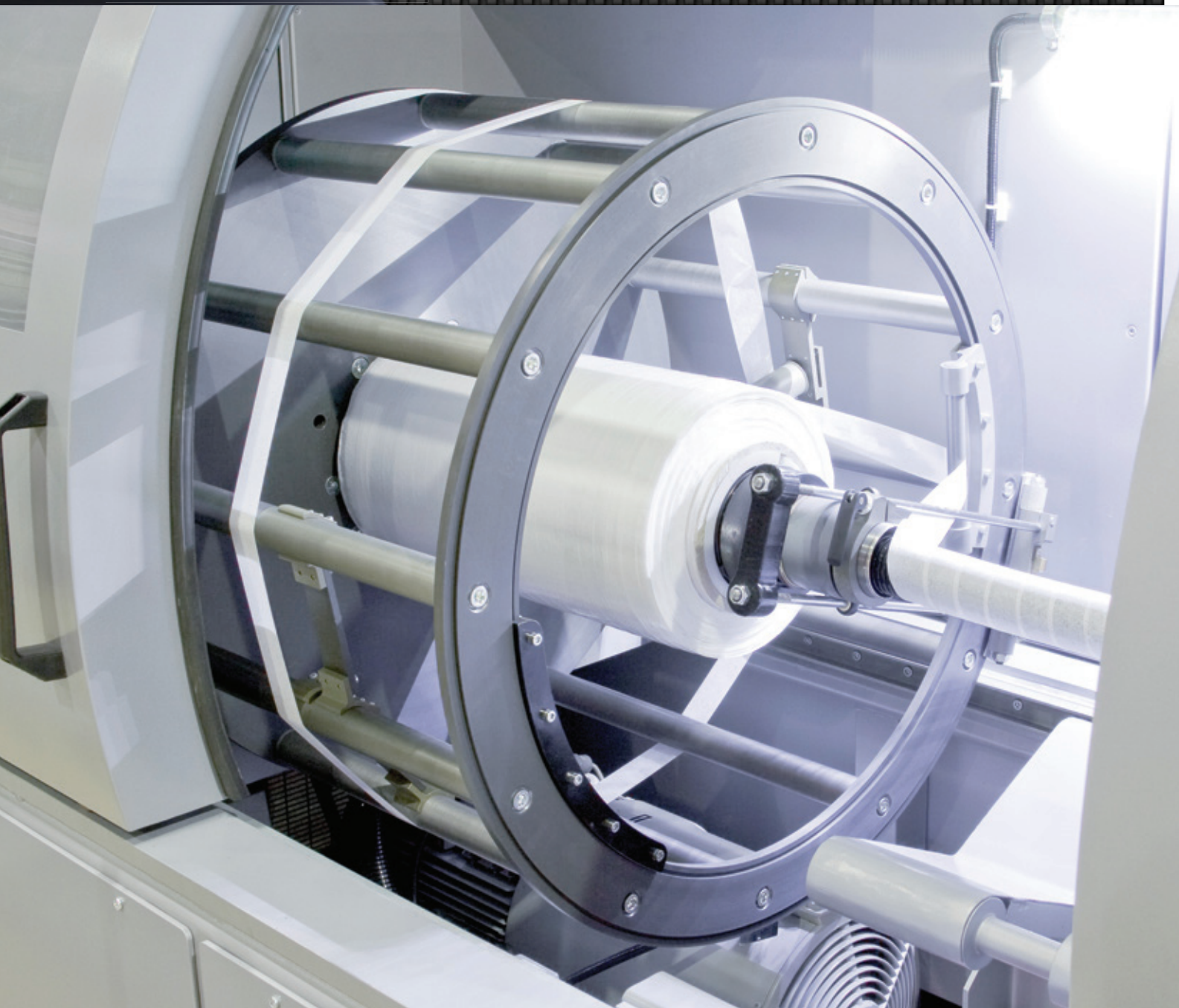
○ Rosendahl's helical tape applicator Rota 500
