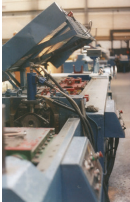
○ Transducer/die assembly fitted to a Schumag drawing machine
