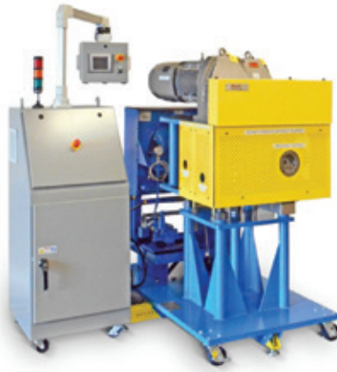
○ The Bullet II, showing the absence of hardware, ie nuts and bolts, so disassembly, cleaning and restart are made easier
