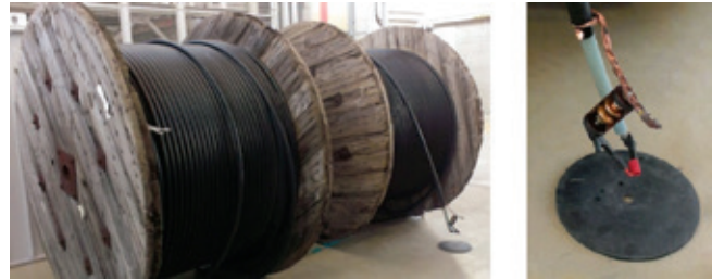
○ Figure 5: AC cable with spark gap (detail)
