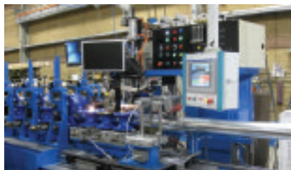
▲ The latest longitudinal metal tape seam welding and corrugating line from Weber & Scher
