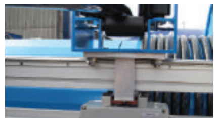
▲ Uhing ARG4-60 rolling ring drive/assembly with load carrier. Photo: Keith Makinson, BAS
